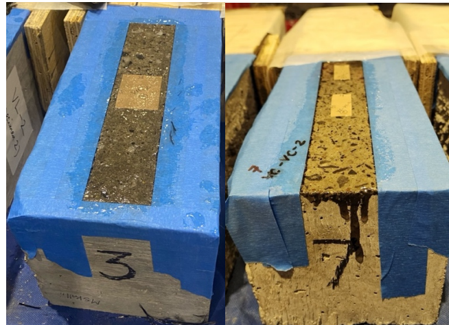
Fig. 3-9. Defect placement during fabrication.
