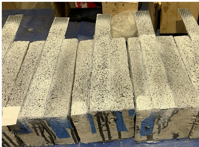
Fig. 3-11. Specimens prepared with white paint and black speckle patterns for 3D DIC acquisition.
