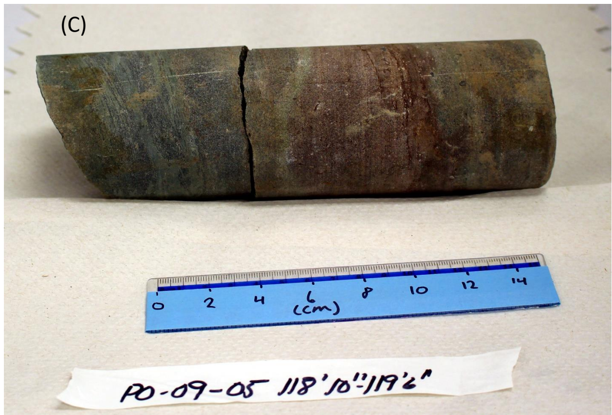
Figure 3.4. Selected core samples from PO-09. A: Red-grey pebble breccia, B: Green-grey mudstone with sand, gravel, and pebbles, C: Multicolored medium sandstone with interbedded clay.
