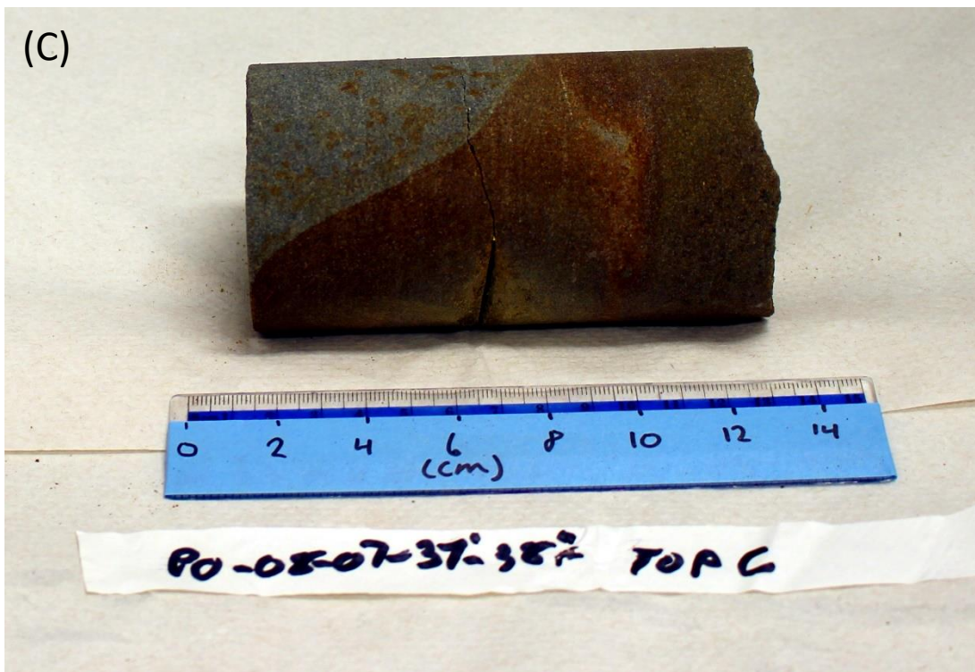
Figure 3.3. Selected core samples from PO-08. A: Grey sandstone, B: Grey sandstone showing bituminous cement C: Sandstone showing transition between red-brown, oxidized zone and grey, reduced zone.
