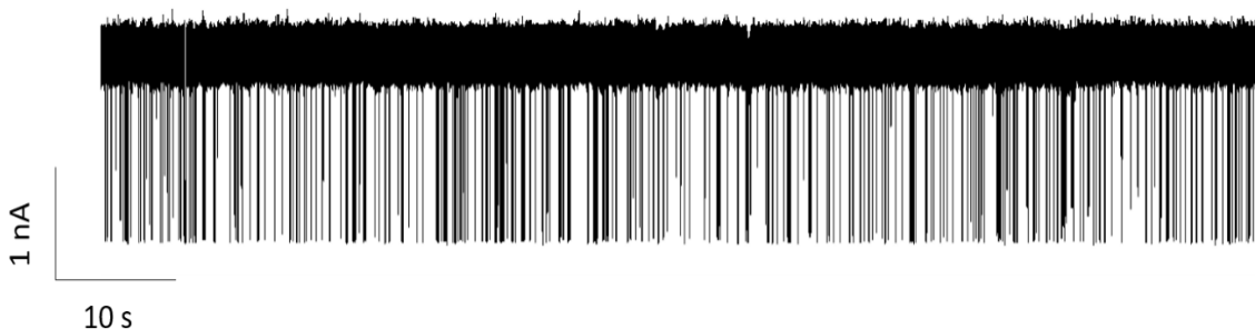
Figure 8. Continuous current trace with 50bp dsDNA in 3.6M LiCl solution under an applied voltage of 300mV.
