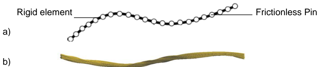
Figure 2.5: Digital element simulation: a) fibre representation b) yarn representation with 19 fibres [118]
