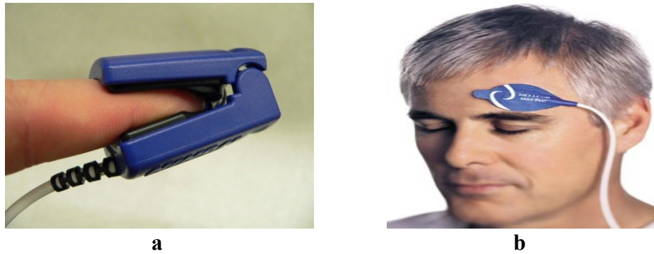
Figure 2.17. The types of oximeter sensors: (a) transmittance configured in a peg model to clip finger. Reproduced from (Wikipedia ® 2013), and (b) reflectance configured oximeter attached to the forehead. Reproduced from (ALLMED ® .Net 2009).
