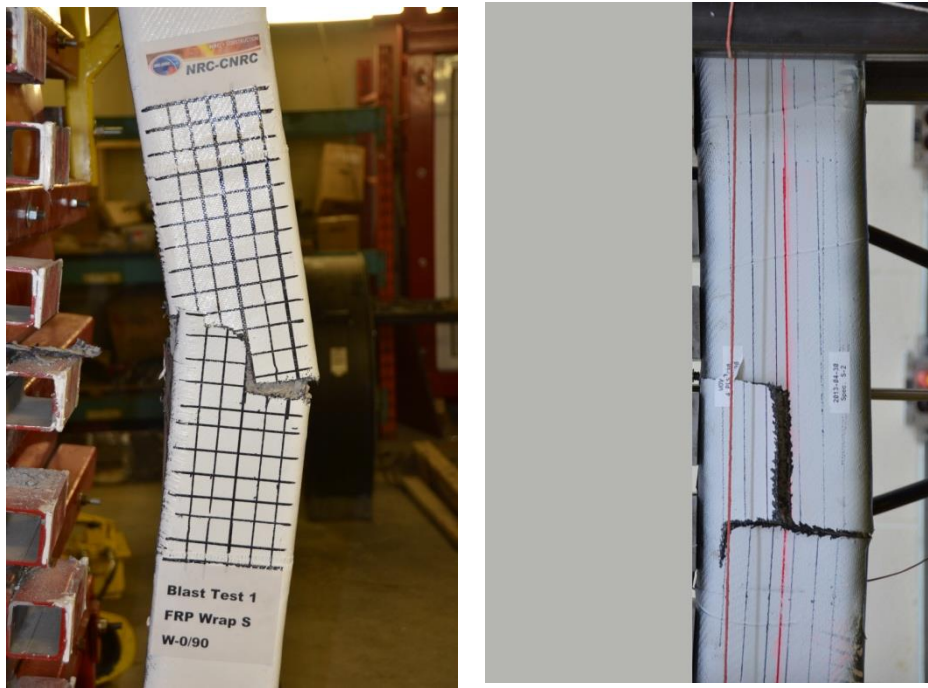
(a) (b) Fig. 5.30 Damage level of S3 - Blast vs. QS
