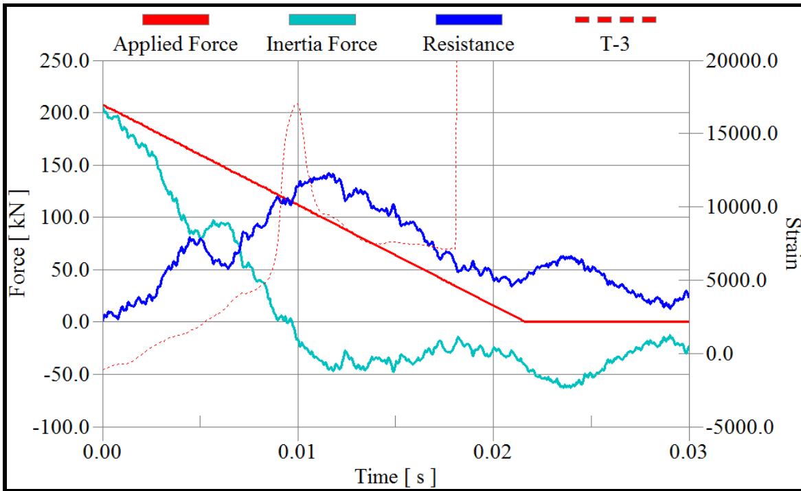
Fig. C-12 Applied force, inertial force, and resistance time history of column S1-C-G1
