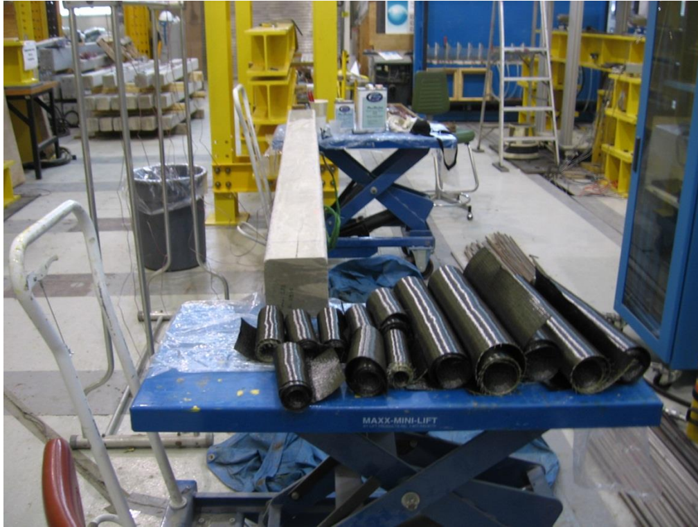
Fig. 3.13 CFRP sheets cut to size
