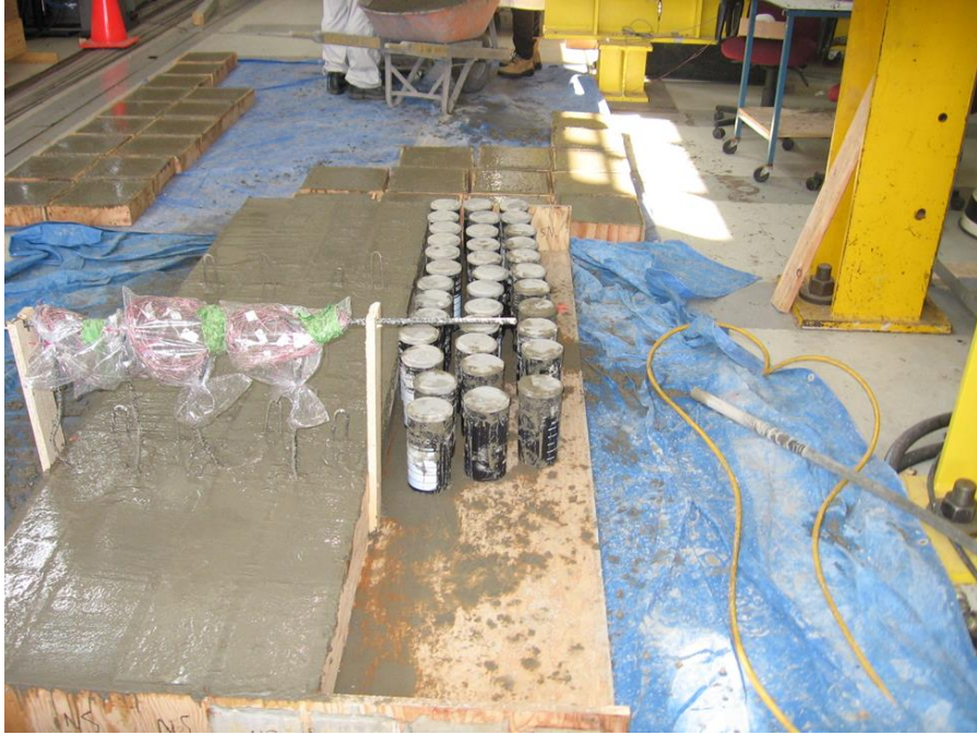
Fig. 3.7 Concrete cylinders preparation
