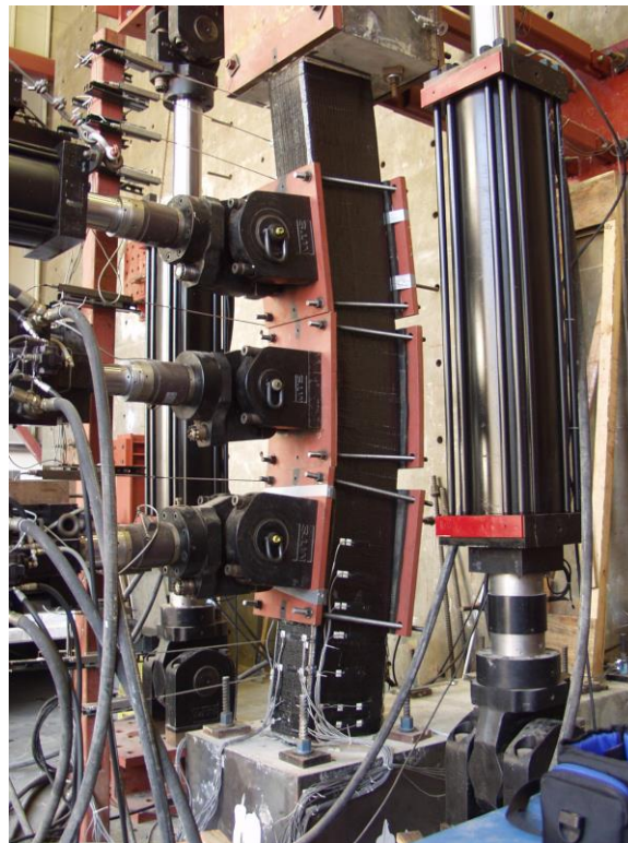
Fig. 2.20 Full scale CFRP RC column tested by lateral loading system (Morris et al. 2004)
