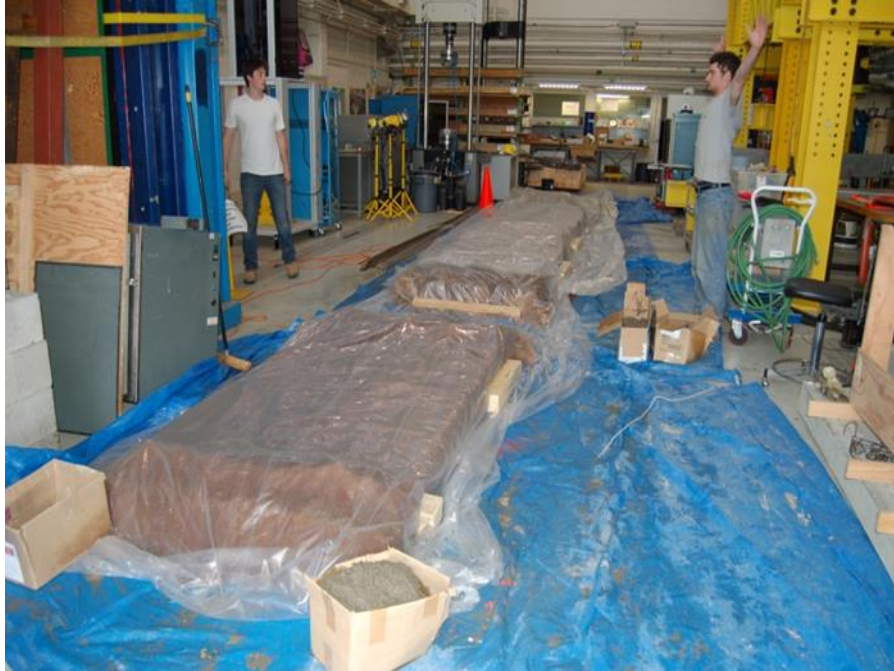
Fig. 3.9 Concrete covered by plastic sheets
