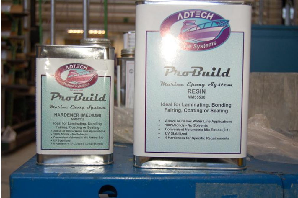
Fig. 3.15 Epoxy resin and hardener used
