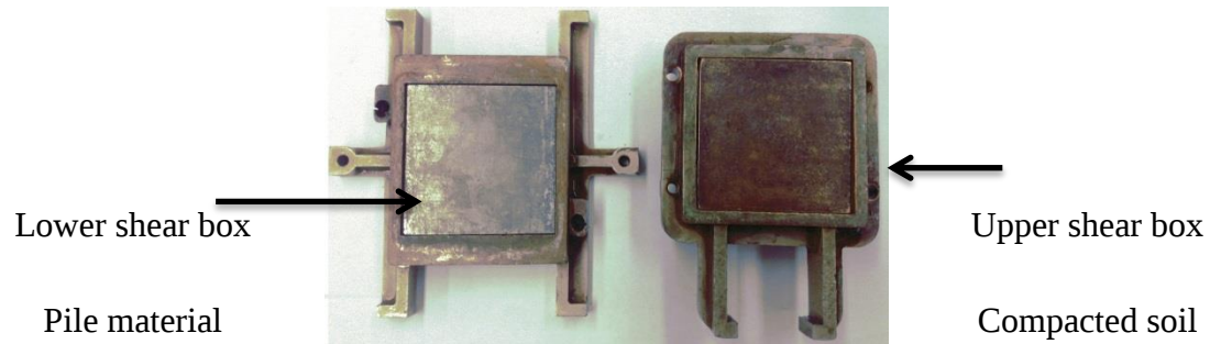
Figure 4.14 Direct shear box interface test
