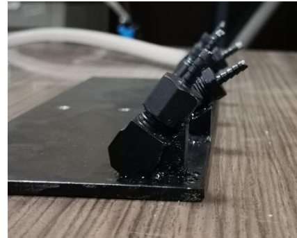
Figure B-5 Designed multiport diffusers with (a) uniform ( 50^\circ ) and (b) non-uniform ( 60^\circ and 40^\circ ) port orientation.
