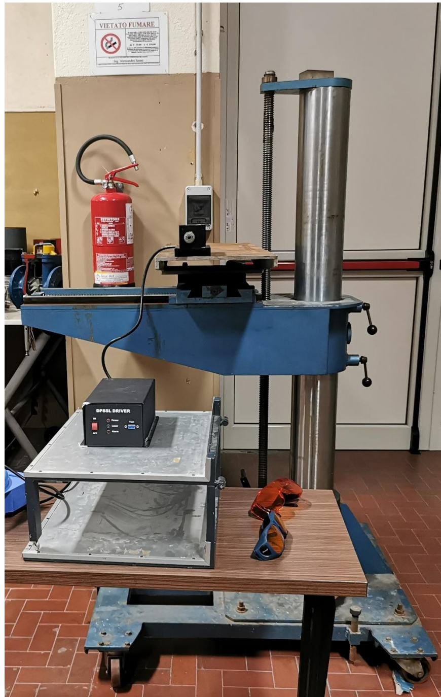
Figure B-7 Tool used to move the laser sheets, showing the laser setup.
