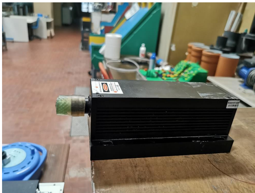
Figure B-3 5-W diode-pumped solid-state (DPSS) continuous green laser.
