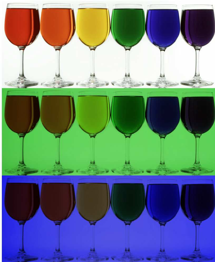
Figure 1.3: Illustration subtractive colour mixing in means of colour filtering, and selective reflection. Wine glasses with rainbow coloured liquids shot against white, green, and blue background. The colour liquids act as optical colour filters pass light of particular wavelength range. The green and blue background themselves selectively reflect light of particular wavelength range. As is observed, subtractive mixing of different colours always reduces the brightness because partial energy is absorbed and/or reflected.
