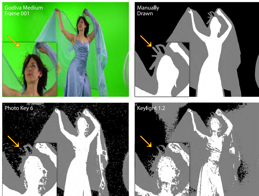
Figure 3.10: The original video frame (top left, the 1 st frame of Godiva medium sequence from [3]), the manually drawn segmentation map (top right), the segmentation map from Photo Key 6 Pro [77] (bottom left), and the segmentation map from Keylight 1.2 [78] (bottom right). Arrows indicate the position of the hardly visible hair.
