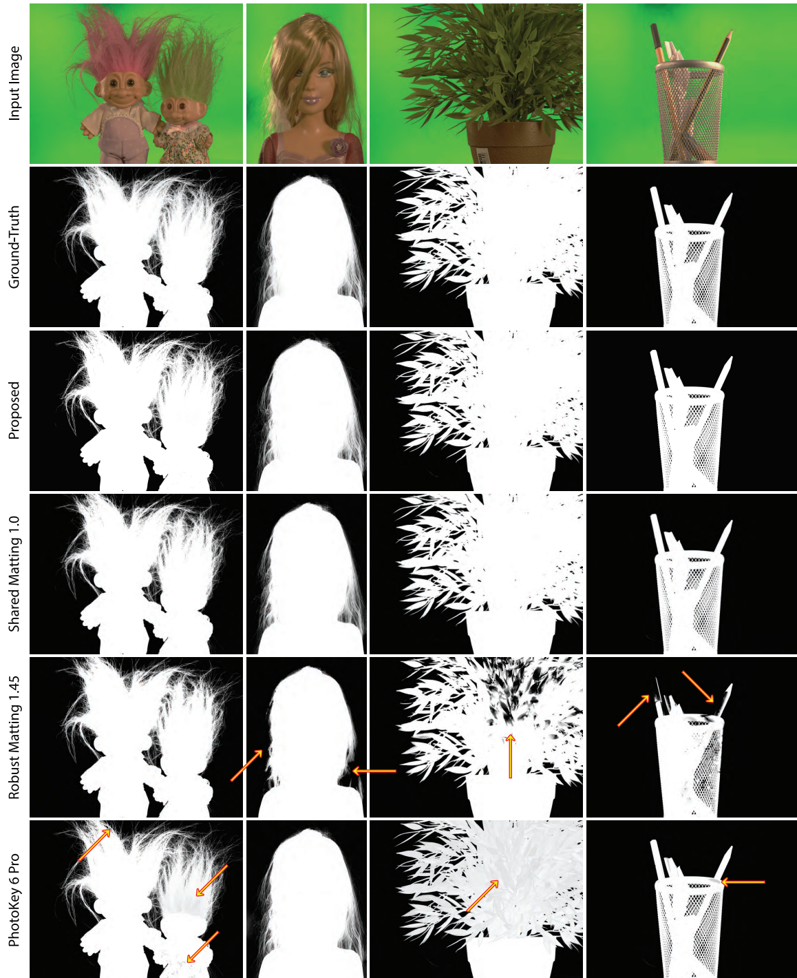
Figure 5.17: Alpha map comparison of quantitative evaluation. From left to right: GT04, GT08, GT13, and GT25. Arrows indicate obvious local flaws.
