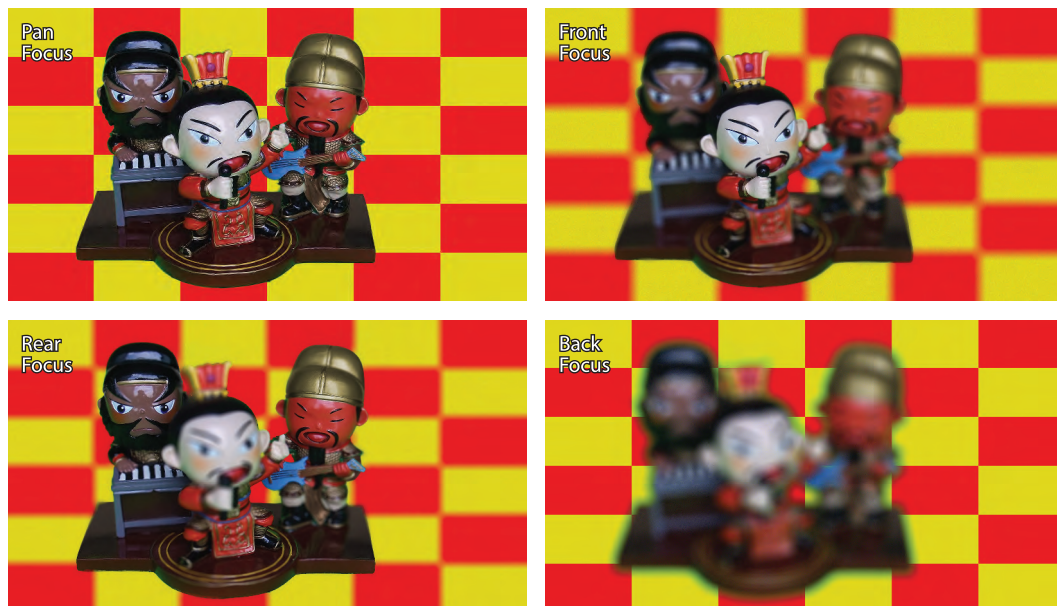
Figure 5.7: Demonstration of depth of field rendering using experimental results. The composite is rendered at different focal lengths.
