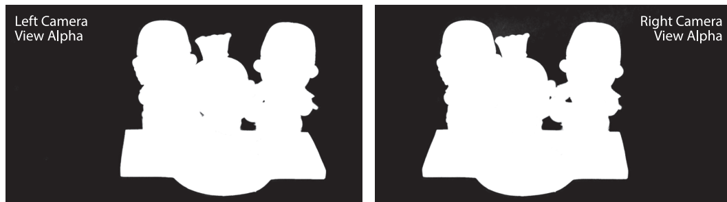
Figure 5.5: Stereoscopic alpha map pair of the 3D chroma keying test scene.
