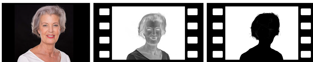
Figure 2.1: Illustration of the Williams’ Process. The foreground is shot against a black background (left) using negative film (middle), and the exposed negative film is intensified during developing to generate the mask (right). For negative films, the latent images were exposed darkens and forms a visible image during developing, the darker the less transparent. The smiling senior woman photo courtesy of Lammeyer [18].
