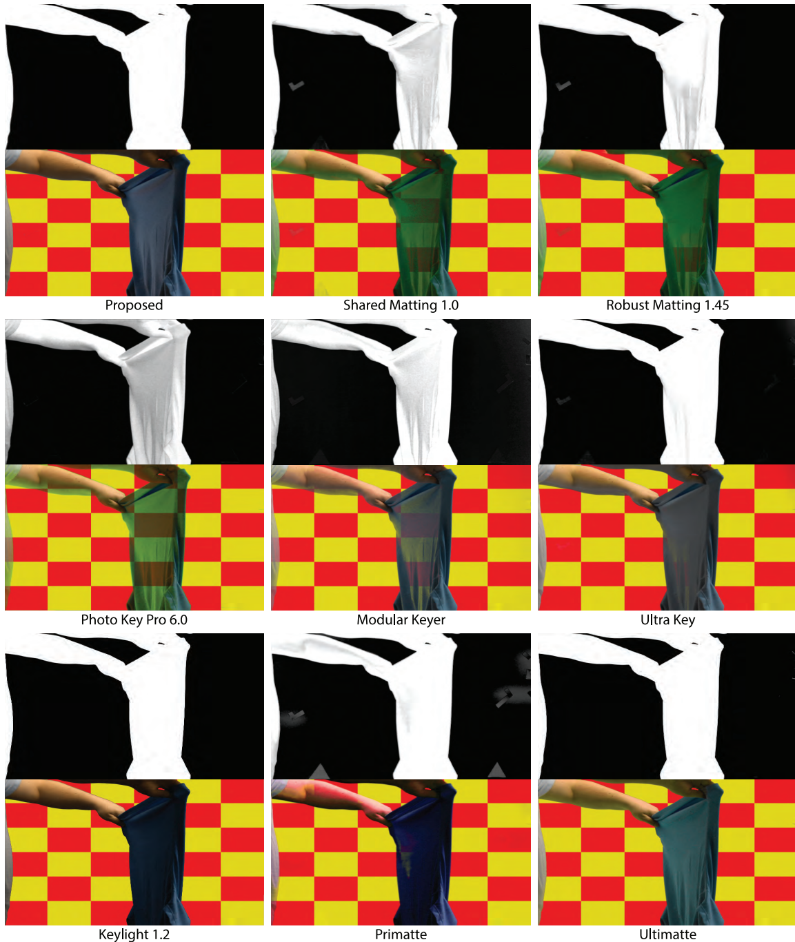
Figure 5.14: Alpha map & foreground comparison of the 44 th frame of the Sheen sequence. In this turn, some traditional chroma-keyers have good results on alpha maps, but the proposed one still have better foreground restoration. It is apparent that there are unwanted colour fringes along the objects' boundary, which is also observed by its publisher [108]. Some software shrinks the matte so that the fringes do not appear in the final result.
