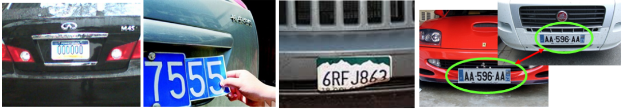
Figure 1.1: (Left-Right) Some cases where detected license plates are ambiguous, forged, damaged, or duplicated, making the license plate recognition based VMMR Systems to fail.
