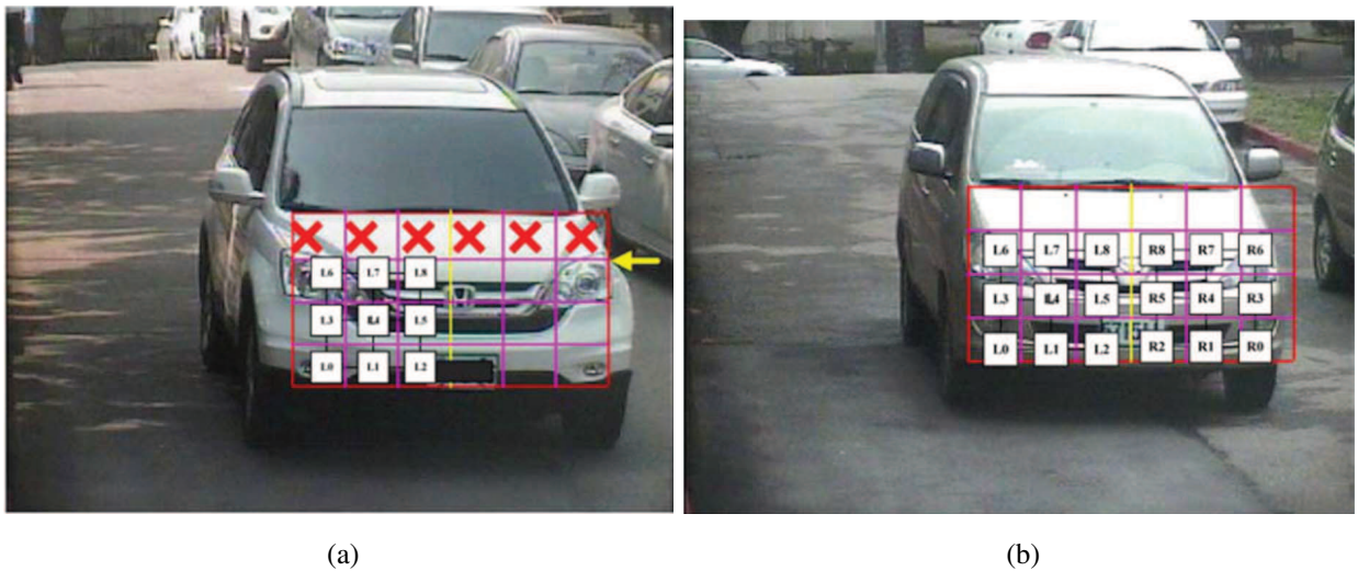
Figure 3.9: Two methods of Inside Division scheme: (a) Symmetrical Inside Division (SID); (b) Full Inside Division (FID). (reprinted from [10])
