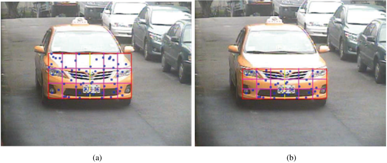
Figure 3.7: Grid-based Representation of vehicle makes and models: (a) Direct Division scheme; (b) Indirect Division scheme. (reprinted from [10])
