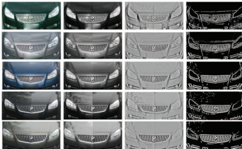
Figure 3.13: He et al.'s features extraction and global representations of vehicle makes and models. (reprinted from [6])
