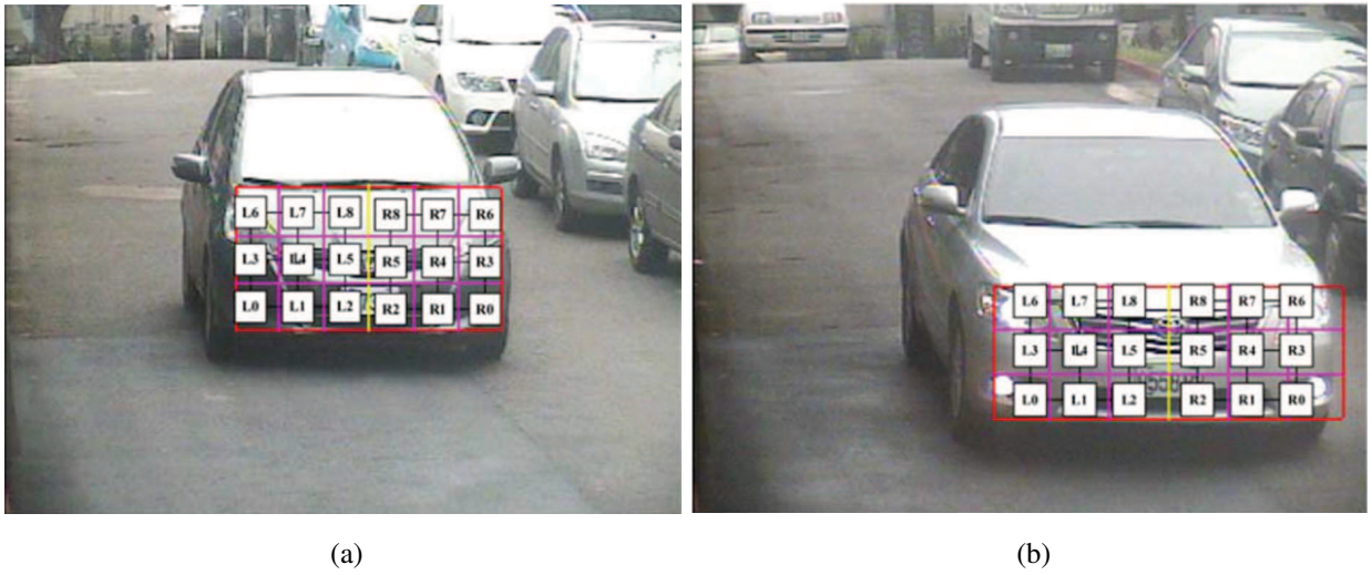
Figure 3.8: Two methods of Direct Division scheme: (a) Wide Direct Division (WDD); (b) Narrow Direct Division (NDD). (reprinted from [10])
