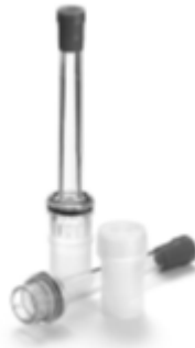
FIGURE 23- CENTRIFREE (R) ULTRAFILTRATION DEVICE USED FOR ASSESSING PLASMA PROTEIN BINDING. IT WORKS BY SEPARATING FREE FROM PROTEIN-BOUND MICROSOLUTES IN SMALL VOLUMES (0.15- 0.1 ML) OF SERUM, PLASMA AND OTHER BIOLOGICAL SAMPLES THROUGH A LOW-ADSORPTIVE HYDROPHILIC MEMBRANE AND USING A METHOD CALLED ULTRAFILTRATION.
