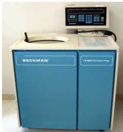
FIGURE 25- BECKMAN L8-70M ULTRACENTRIFUGE USED FOR CENTRIFUGING HOMOGENIZED RAT KIDNEY TISSUE DURING METABOLISM STUDIES.
