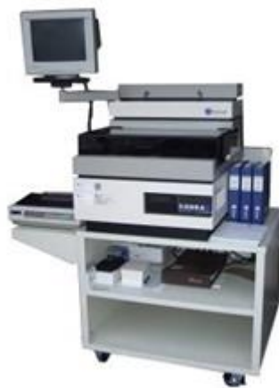
FIGURE 21- THE PERKIN-ELMER (PACKARD) COBRA II GAMMA COUNTER.
