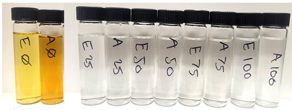
Figure S 4.3. The appearance of solutions containing 0.2 mM \text{AgNO}_3 , 1 mM citrate, and 0.2 mM of either I-2959 (“A”) and I-184 (“E”) as initiators, in mixtures of MeCN and \text{H}_2\text{O} (0%, 25%, 50%, 75% and 100% MeCN) following 15 minutes of irradiation with in a photoreactor with 6, 8W UVA lamps (for the 0% MeCN samples). The samples containing MeCN showed no change after 15 minutes. The MeCN containing samples were subsequently irradiated for a total of 90 min but still did not yield any AgNPs.
