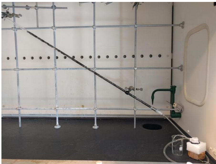
Figure S 2.5. 150 cm length glass tube tilted at around 30°. A miniature peristaltic pump was used for this experiment.
