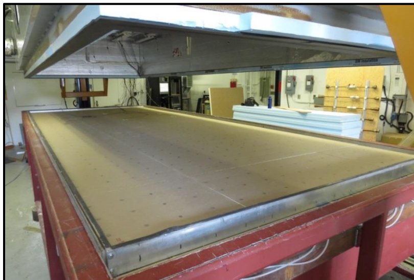
Figure 6-2: Calibrated Thermal Chamber – Polyiso R31 System – No Gaps
