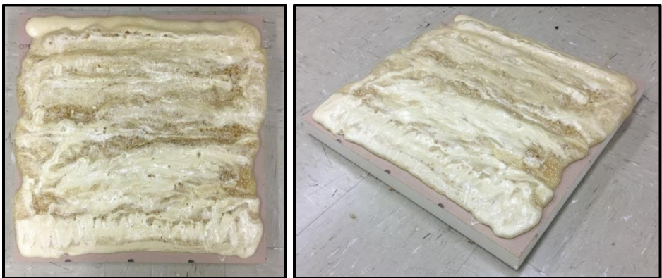
Figure 5-17: Spread Applied Adhesive
