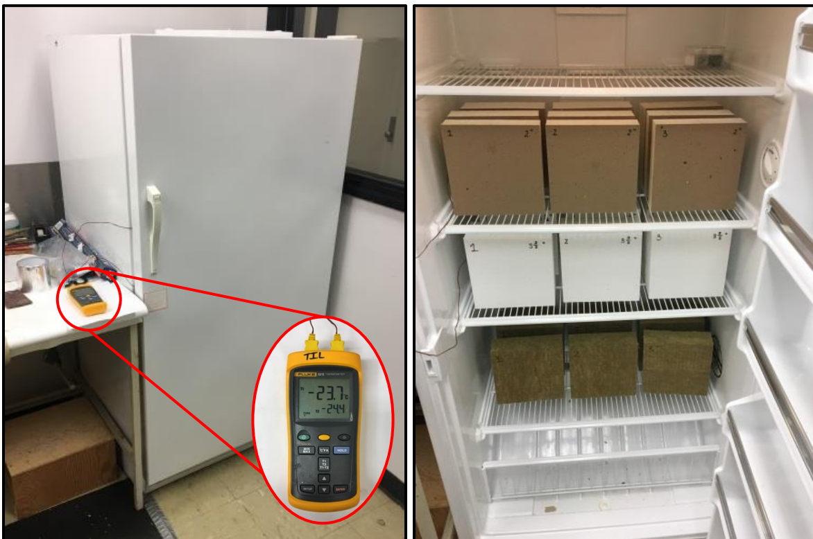
Figure 4-12: Dimensional Stability – Cooling Chamber
