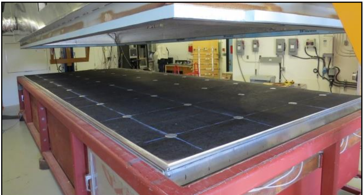
Figure 6-9: Calibrated Thermal Chamber – Polyiso R31 System - Fasteners
