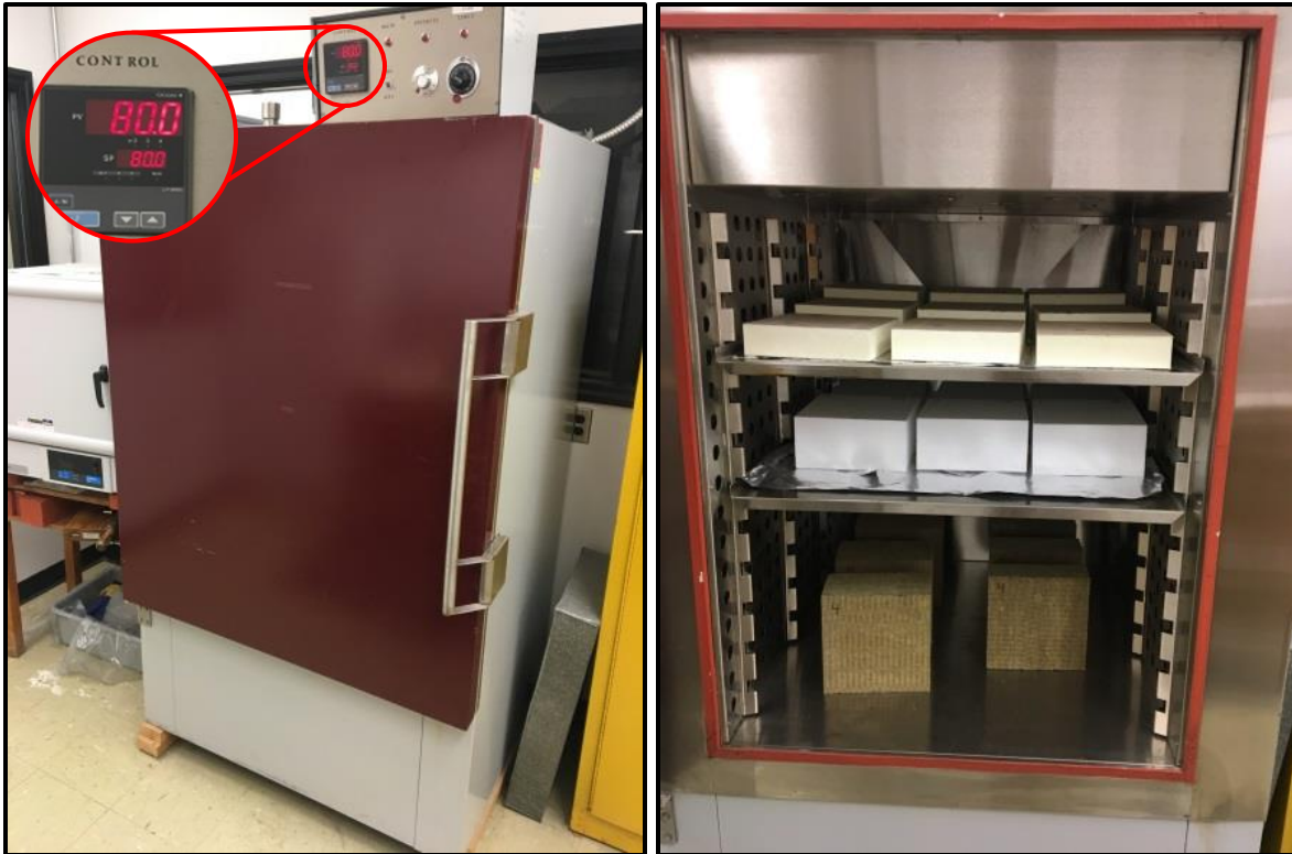
Figure 4-11: Dimensional Stability – Heating Chamber
