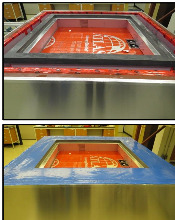
Figure 4-19: Assembled Guarded Hot Box
