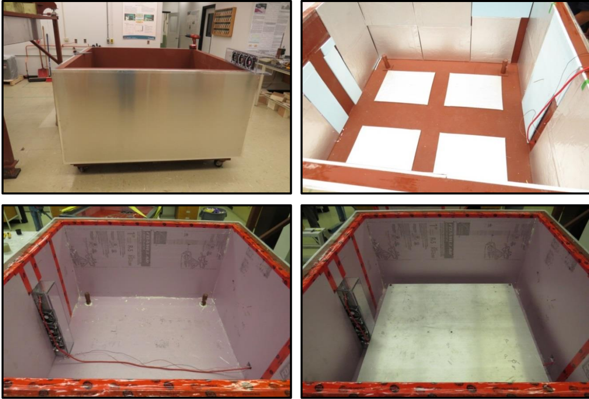
Figure 4-16: Insulating the Walls of the Guard Chamber
