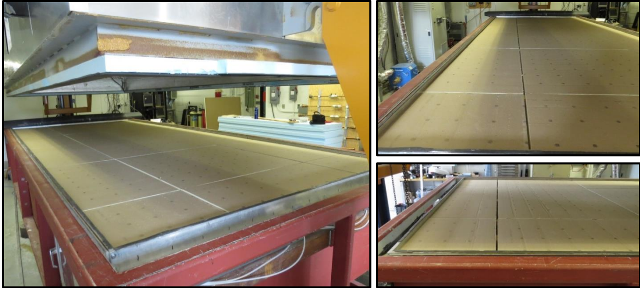
Figure 6-3: Calibrated Thermal Chamber – Polyiso R31 System – ½” Gaps
