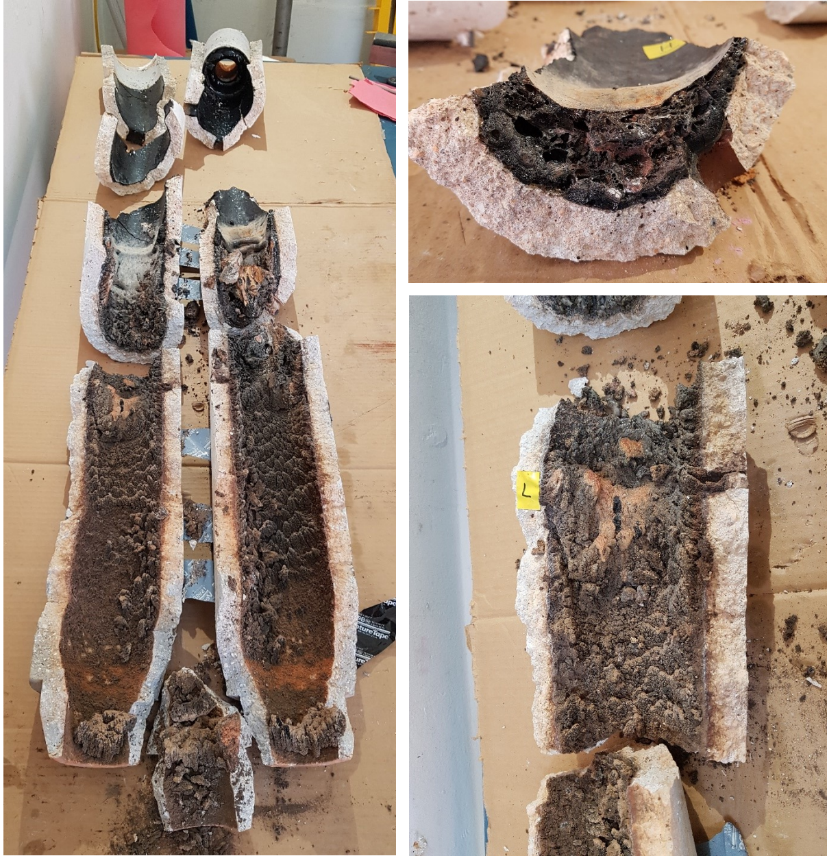
Figure 3-3. Refractory lining (0.1 m ID) of DCSG combustor following a pilot-scale test with MFT-OPW. Combustor conditions: 1100-1250 °C, 55 bar(g), 240 kW. Test duration was 100 min.
