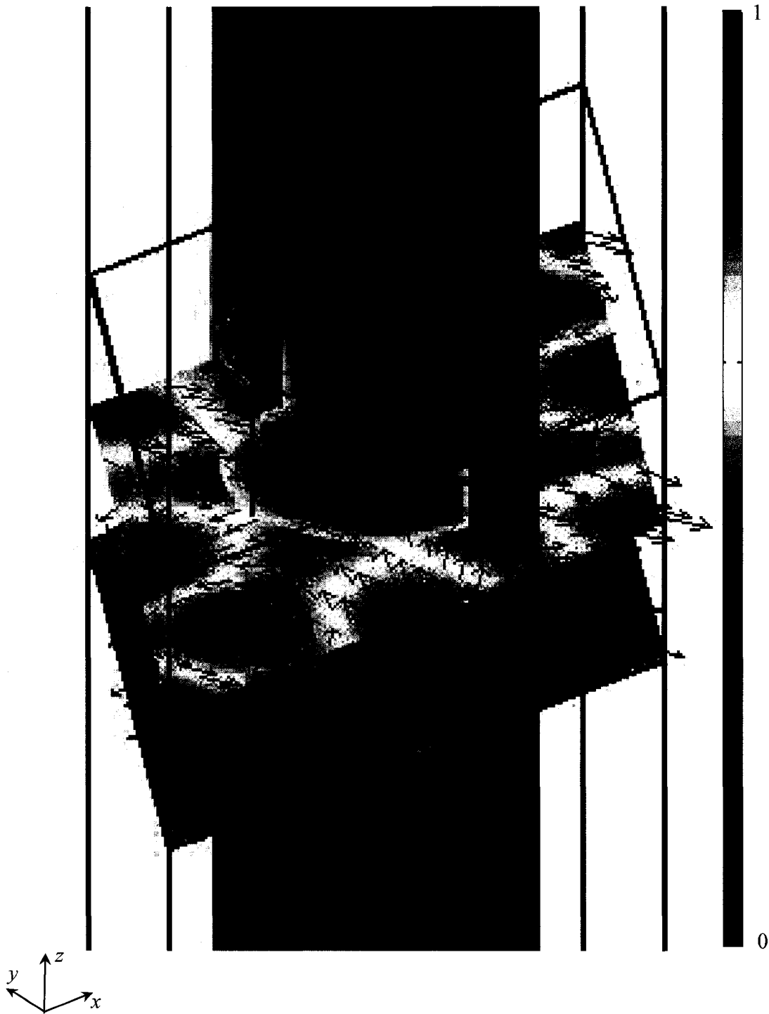
Figure 34. Hexagonal photonic crystal slab lattice air holes in dielectric background Bloch mode, band 1, \mathbf{k} = \hat{\mathbf{x}} 4\pi/(3a) Poynting vector magnitude and direction (arrows) three-dimensional view. Bold lines represent the edges of the photonic crystal slab unit cell.
