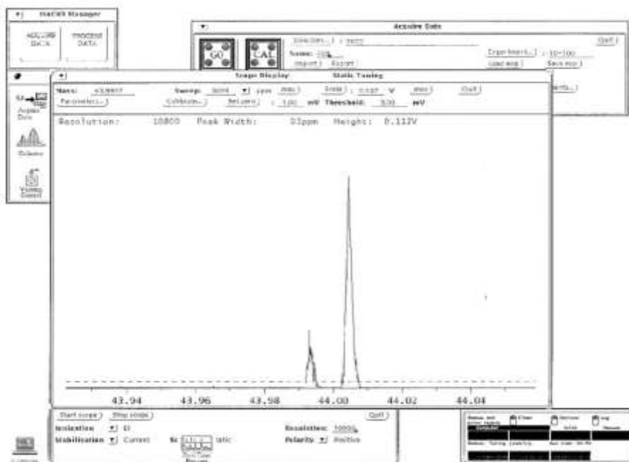
Figure E.1. Mass spectrum of gas products after CPE experiment shown in Table 7.2, row 7. The peak at 30.0 shows NO gas and the peak at 44.01 shows N 2 O gas.
