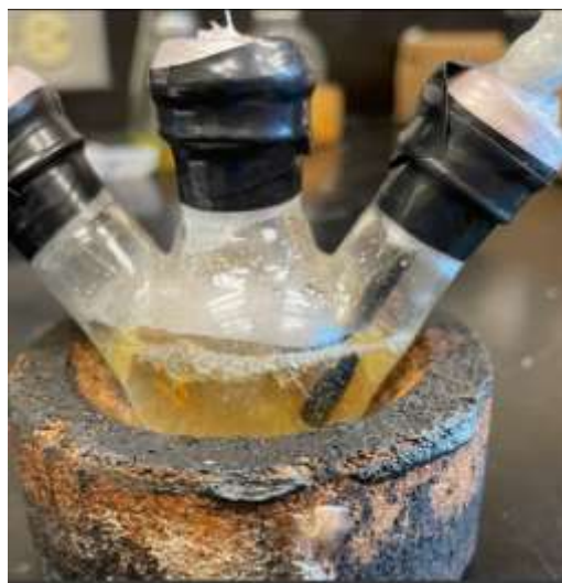
Figure 4.25. Produced \text{H}_2 gas bubbles in the electrochemical cell after CPE shown in Table 4.4, row 1.
