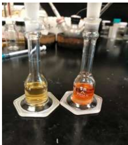
Figure 6.25. Sample solution color before (left) and after (right) hydroxylamine test.
