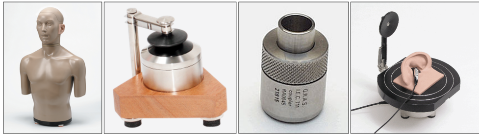
Figure 4.1: Devices used to measure noise levels under communication headsets. a) KEMAR acoustic manikin - G.R.A.S., 45BA - (Permission to reproduce this image was granted from G.R.A.S.), b) Type 1 artificial ear - Brüel & Kjaer, 4153 - (Copyright © Brüel & Kjaer), c) Type 2 artificial ear - G.R.A.S., RA0045 - (Permission to reproduce this image was granted from G.R.A.S.), and d) Type 3.3 artificial ear - G.R.A.S., 43AG - (Permission to reproduce this image was granted from G.R.A.S.).
