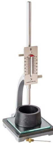
Figure 2.3 Vicat apparatus used to determine the initial and final setting times of CPB. Source: Forney CMT Equipment (n.d.).
