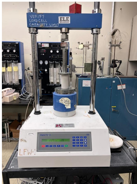
Figure 2.4 Uniaxial compressive strength (UCS) testing machine used to measure the compressive strength of CPB specimens. Source: Laboratory of Dr. Fall, University of Ottawa.
