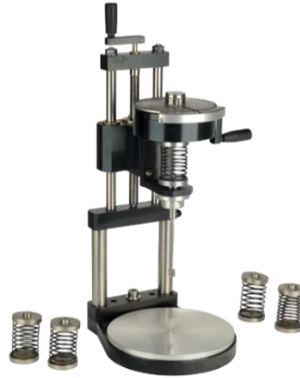
Figure 2.2 Laboratory vane shear apparatus (Wykeham-Farrance) used to determine the yield stress of CPB. Source: VJ Tech Limited (n.d.).
