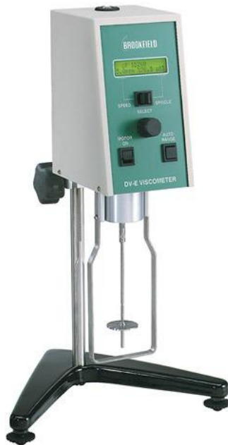
Figure 2.1 Brookfield digital viscometer (DV-E model) used to measure the viscosity of CPB samples. Source: LABOMAT ESSOR SA (n.d.).
