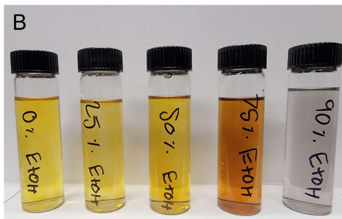
Fig. 2.1.54: A) UV-Vis spectra of AgNPs synthesized in batch scale, using 0.2 mM I-2959 as an initiator. Solutions were prepared in mixtures of EtOH/H 2 O in ratios ranging from 0 to 90% EtOH, and irradiated for 15 min in a photoreactor with 6 8W UVB lamps. The 90% EtOH sample was irradiated for an additional 25 mins, as little color could be seen after 15 min of irradiation. B) Corresponding appearance of AgNPs produced in solutions containing different fractions of EtOH following reacting under UVB.
