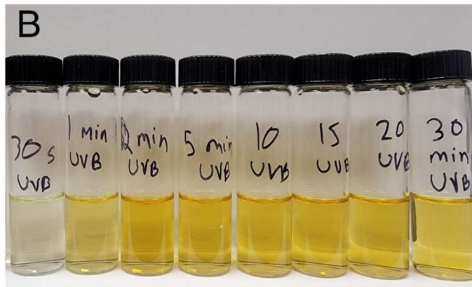
Fig. 2.1.S5: A) UV-Vis spectra of AgNPs synthesized in single batches, using 0.2 mM I-2959 in H 2 O. Samples were irradiated in a photoreactor with 6 UVB lamps for 30 sec to 30 min to determine the endpoint of the reaction. B) The appearance of the corresponding nanoparticle suspensions.
