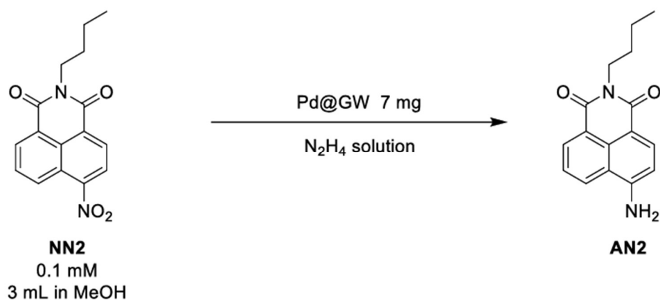
Scheme 5.1.S5: Reduction of the fluorogenic probe NN2 by Pd@GW using N 2 H 4 .
