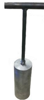
(E) Photo of compaction hammer
