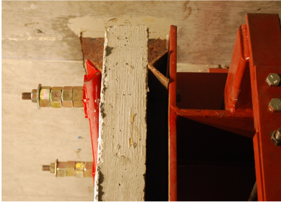
Figure 3.14: Close-up of Back-to-Back Angles Used for Knife Edge Supports in Companion Set 3 and 4.
