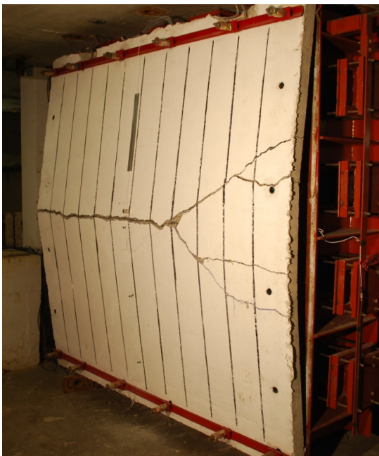
(c) After shot 3 P_r = 100.6 \text{ kPa} I_r = 811.2 \text{ kPa-ms}
