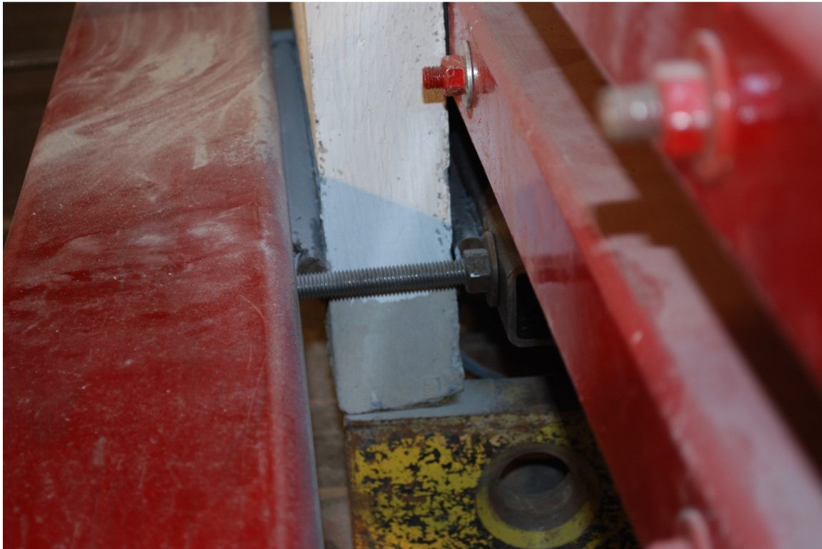
Figure 3.12: Close-up of Support Conditions for Companion Set 1 and 2.
