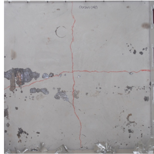
(c) Rebound face After shot 6 P_r = 95.7 \text{ kPa} I_r = 1374.7 \text{ kPa-ms}
