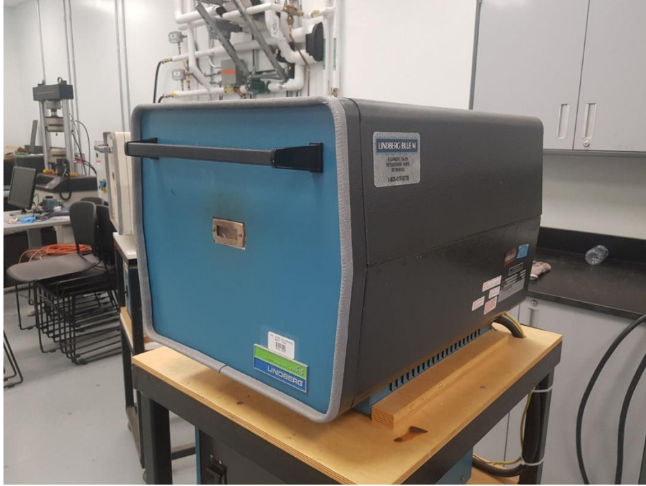
Figure 4.33: Lindberg furnace used for annealing of the copper coatings and fins.
