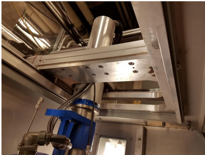
Figure 4.8: CGDS traverse system.
