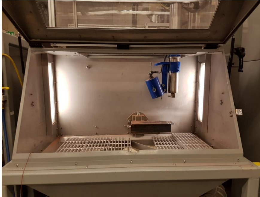
Figure 4.11: CGDS spray chamber.
