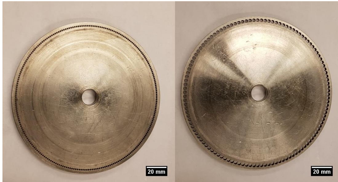
Figure 4.10: 240 medium hole feeder wheel (left), and 120 large hole feeder wheel (right).
