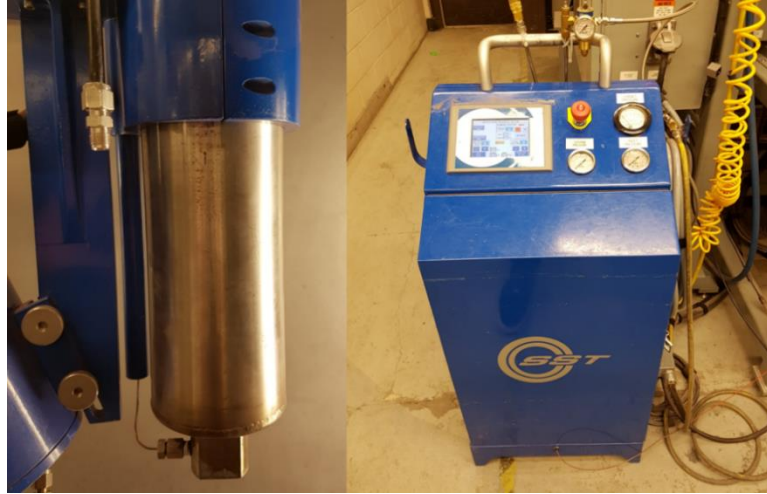
Figure 4.3: CGDS gas heater (left) and control cabinet (right).
