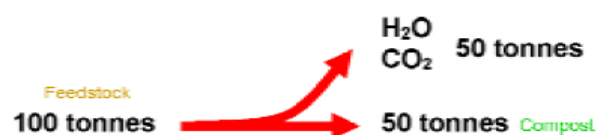
Figure 2.7: Mass balance of composting process (MWIN, 2006).
