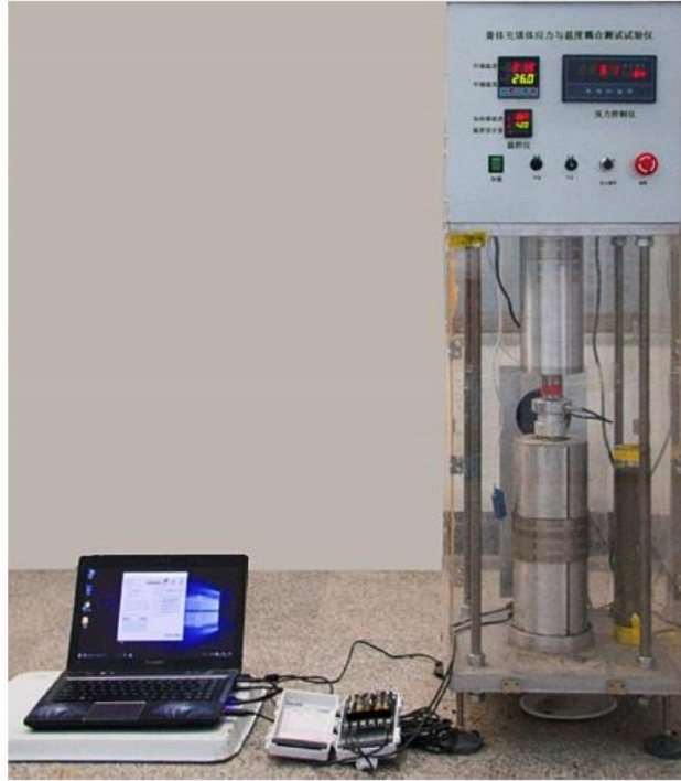
Figure 2.25 Curing under-stress apparatus for assessing the mechanical strength of CPB (Chen et al. 2022)
