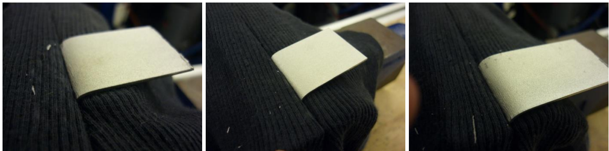
Figure 6.50: Aluminum 7075 strip rupture samples bent to 90° (coating on aluminum IVD coating).
