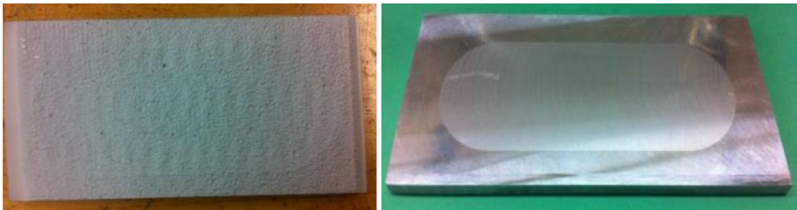
Figure 6.23: Pure aluminum repair before machining (left) and after machining (right).
