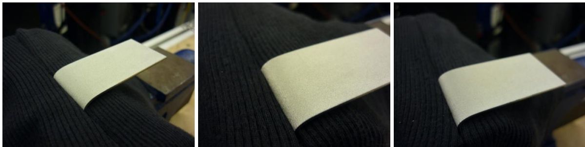
Figure 6.46: Aluminum 7075 strip rupture samples bent to 90° (coating on bare steel).
