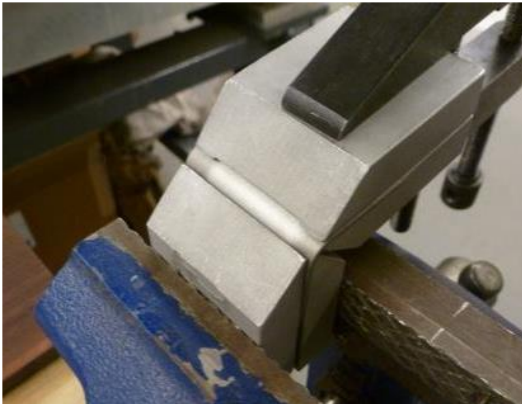
Figure 6.64: Al 7075 Coating Showing No Delamination when Bent to 90 Degrees
