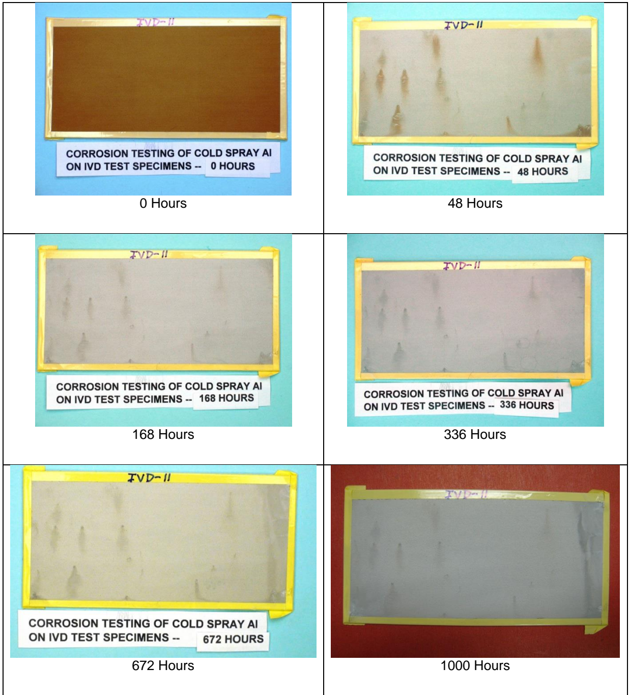
Figure AIV.11: Full corrosion results for aluminum 5083 restoration of damaged aluminum IVD coating (Sample 11).
