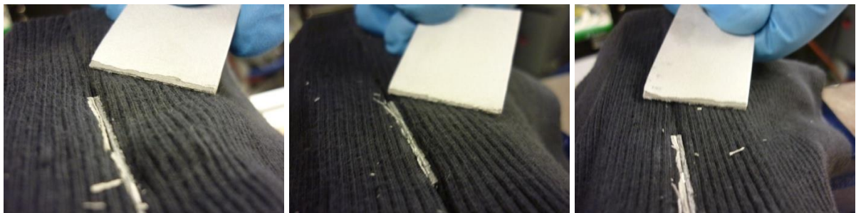
Figure 6.51: Aluminum 7075 strip rupture samples after rupture (coating on aluminum IVD coating).
