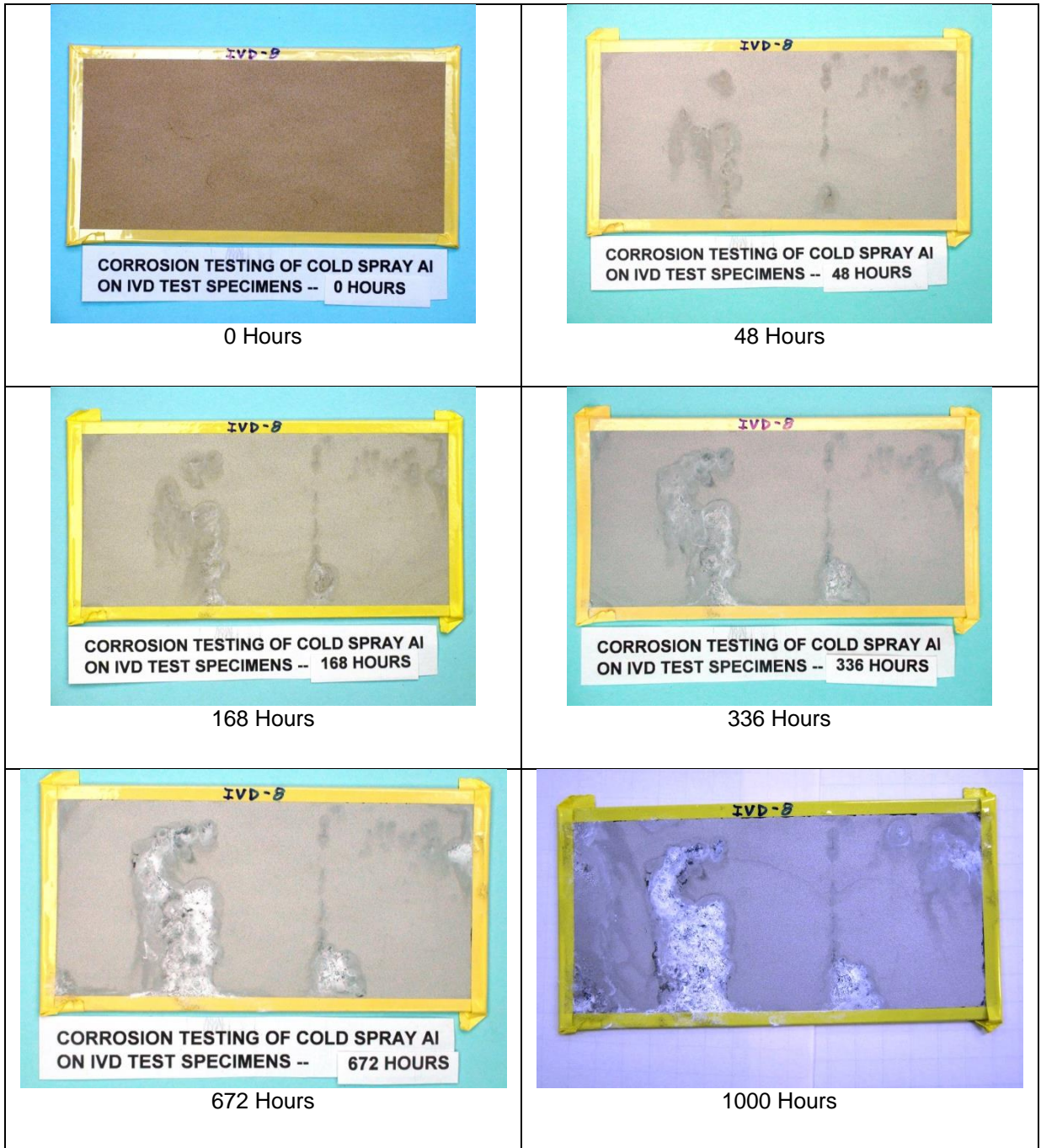
Figure AIV.8: Full corrosion results for aluminum 7075 restoration of damaged aluminum IVD coating (Sample 8).
