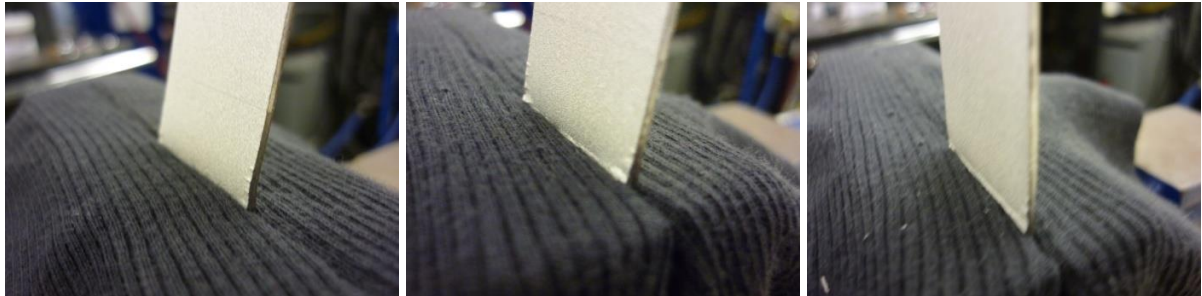
Figure 6.47: Aluminum 7075 strip rupture samples returned to 0°, showing delamination at the edges (coating on bare steel)
