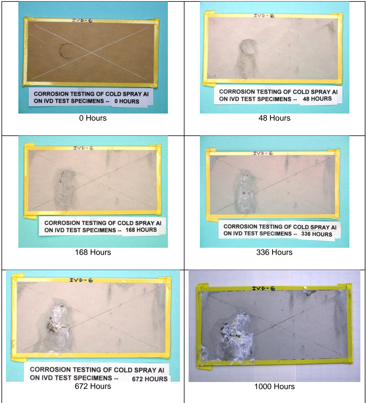
Figure AIV.6: Full corrosion results for aluminum 7075 restoration of damaged aluminum IVD coating (Sample 6).
