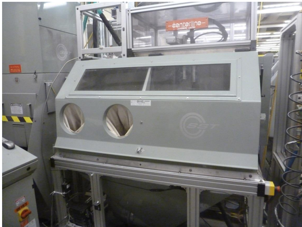
Figure 4.12: Centerline (Windsor) Ltd custom built spray chamber.
