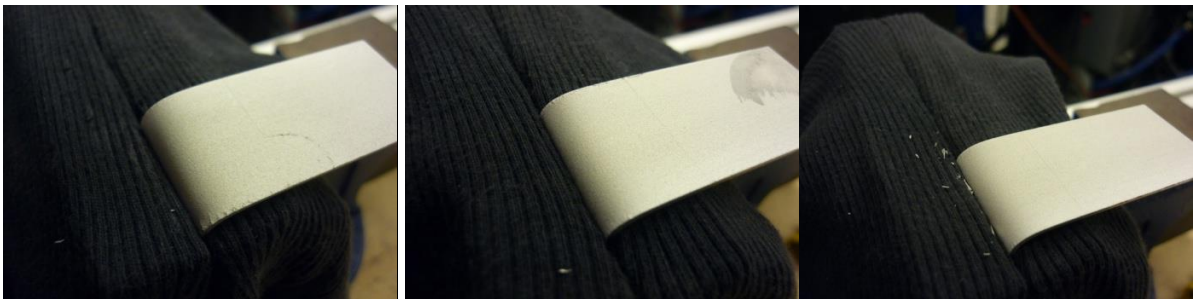
Figure 6.53: Aluminum 5083 strip rupture samples bent to 90° (coating on bare steel).
