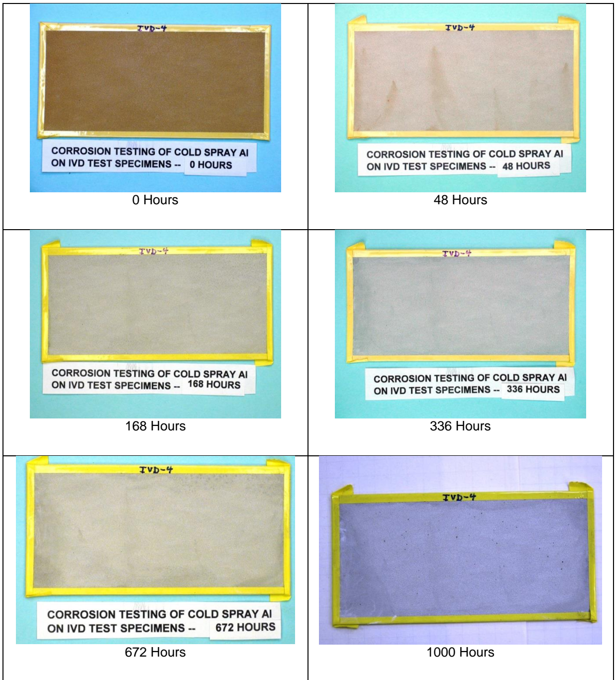
Figure AIV.4: Full corrosion results for pure aluminum restoration of damaged aluminum IVD coating (Sample 4).
