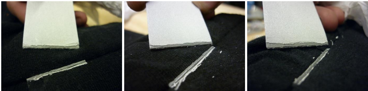
Figure 6.41: Pure aluminum strip rupture samples after testing (coating on bare steel)
