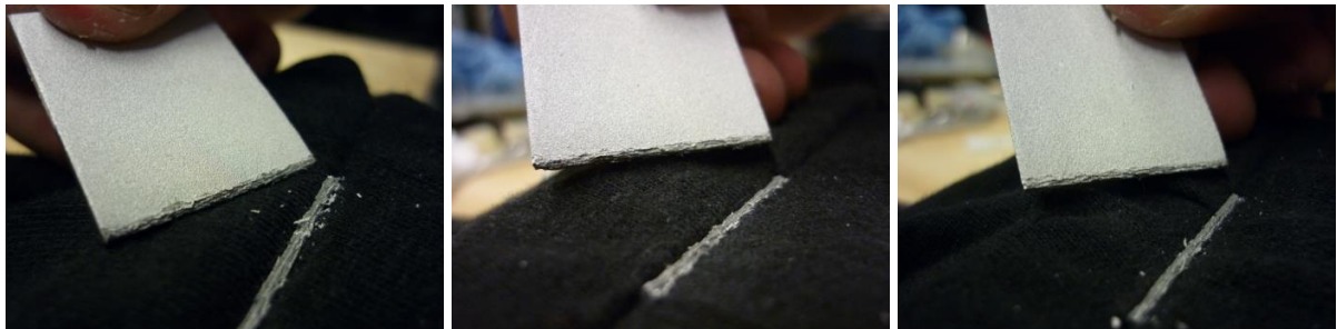
Figure 6.44: Pure aluminum strip rupture samples after rupture (coating on aluminum IVD coating).
