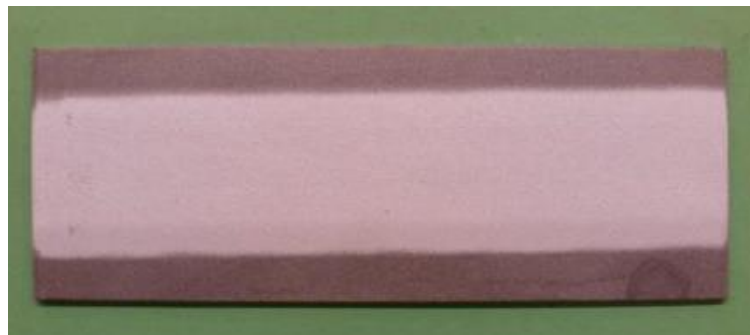
Figure 6.58: Modified strip rupture panel showing coating in the middle.
