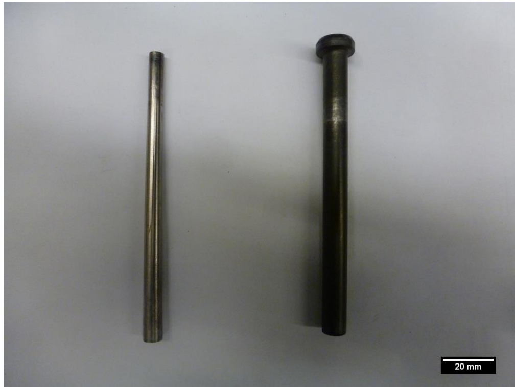
Figure 4.7: Image of stainless steel nozzle (left) and polymer nozzle (right) from Centerline (Windsor) Ltd.
