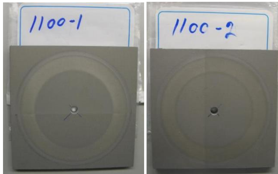
Figure 6.7: Pure aluminum Taber abrasion panels after testing.
