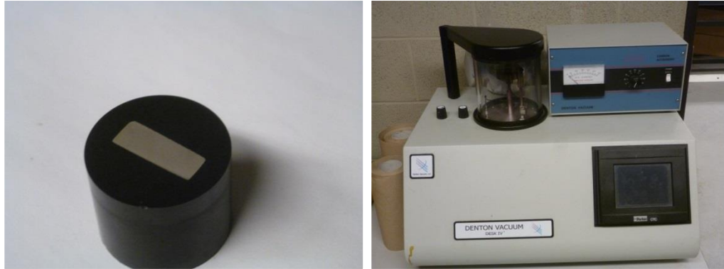
Figure 4.16: Mounted and polished sample (left) and Denton Vacuum Desk IV gold sputtering machine (right).
