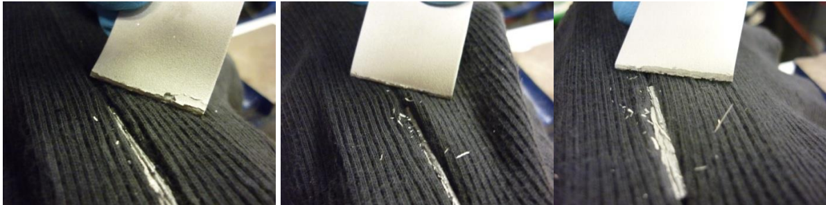
Figure 6.57: Aluminum 5083 strip rupture samples after rupture (coating on aluminum IVD coating).
