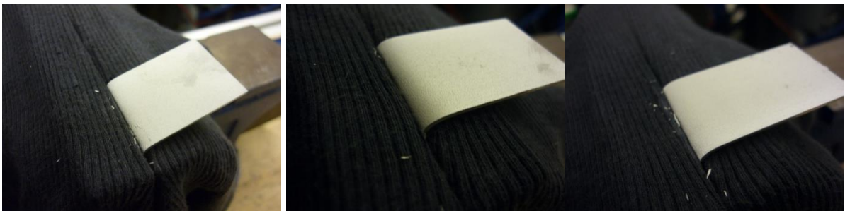
Figure 6.56: Aluminum 5083 strip rupture samples bent to 90° (coating on aluminum IVD coating).
