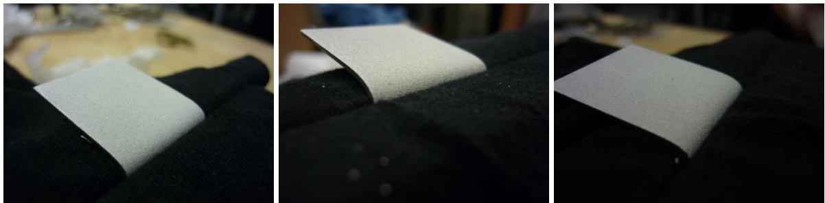
Figure 6.43: Pure aluminum strip rupture samples bent to 90° (coating on aluminum IVD coating).
