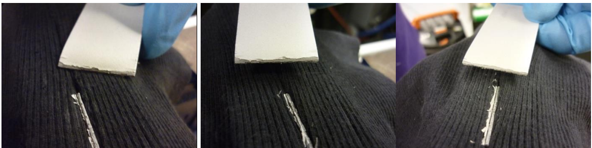
Figure 6.54: Aluminum 5083 strip rupture samples after testing (coating on bare steel).
