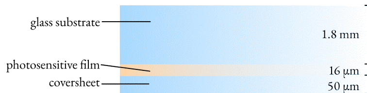
Figure 6.4: Dimensions of the litiHolo C-RT20 photosensitive film procured from ©Liti Holographics [96].
