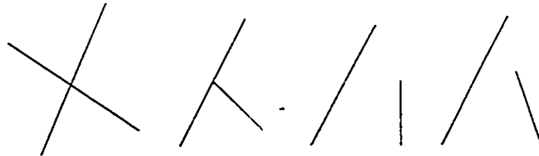
Figure 5.2: Testing whether line segments intersect: four cases.
