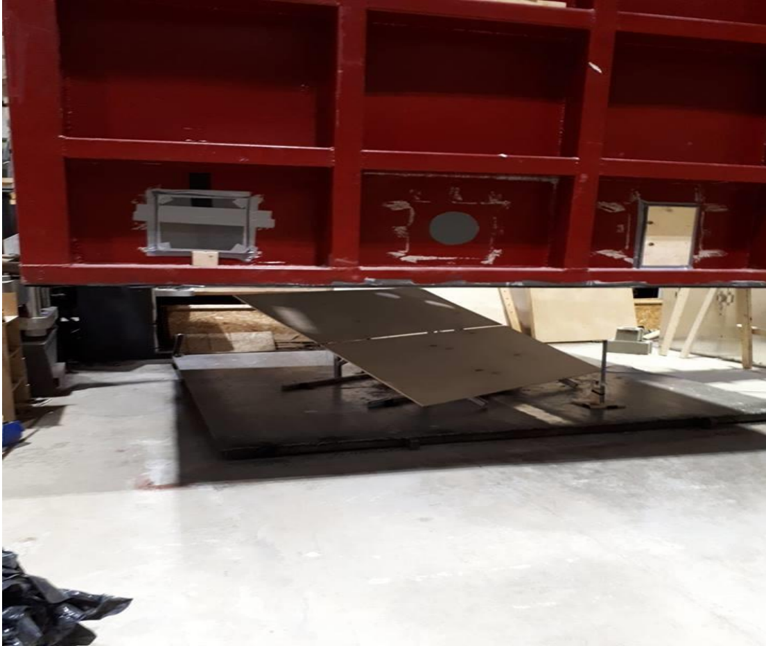
Figure 3.8 Box lifted over the panels by the crane (45° AOI case)
