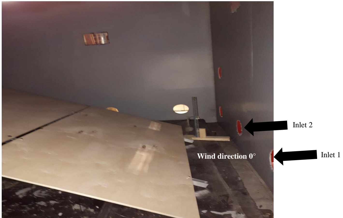
Figure 4.2 Inside view of the WDS with panels inside ( 0^\circ wind angle of incidence)
