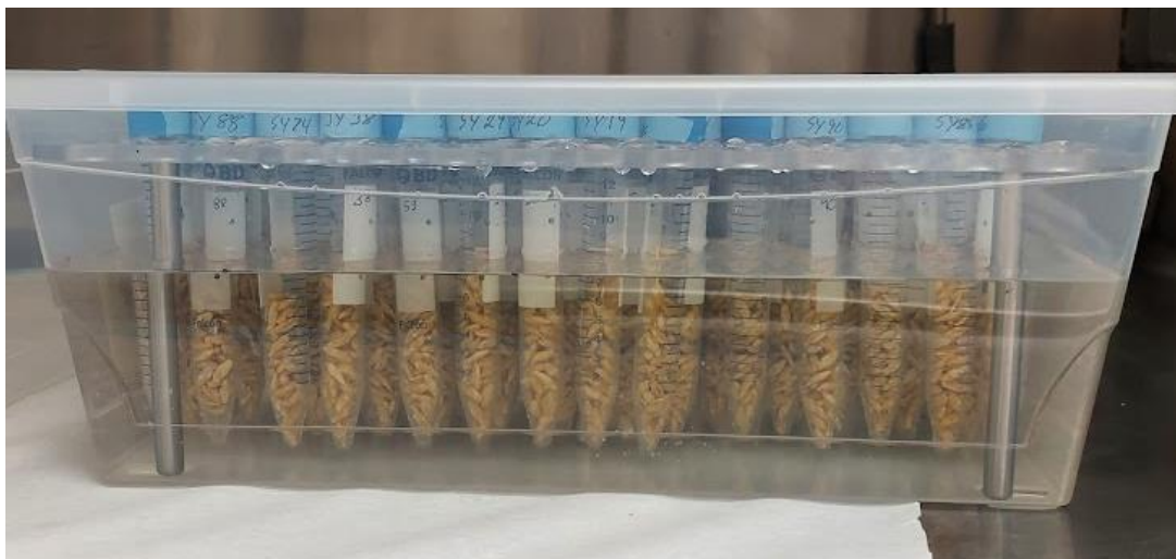
Figure S0.4 Seed sterilization rack developed for simultaneous large scale sterilisation.
