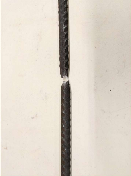
Figure 3.2 - Ruptured No. 4 MMFX® steel bar
