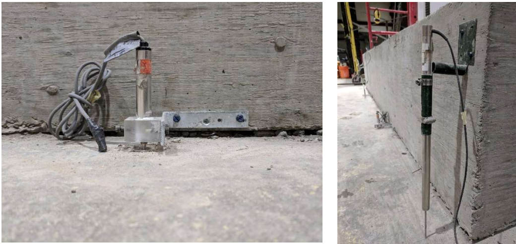
Figure 4.15 - LVDTs installed along the length of the foundation to monitor uplift
