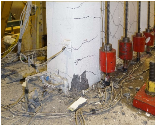
c) West side boundary element at test end
