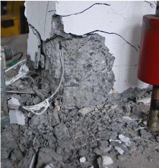
a) West side boundary element at test end
