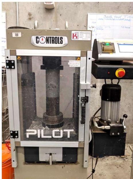
a) Concrete testing cylinder test equipment
