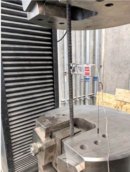
Figure 3.1 - Typical steel bar coupon test setup
