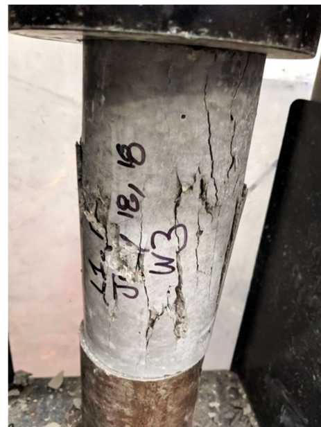
b) Typical concrete cylinder at the end of testing
