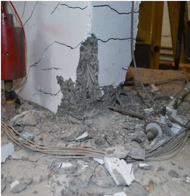
b) East side boundary element at test end
