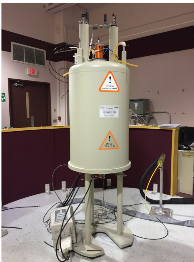
Figure 9. A 9.4 T NMR spectrometer magnet for the solid state. The superconducting coil is found within the large cylindrical container, which also houses the cooling liquid.
