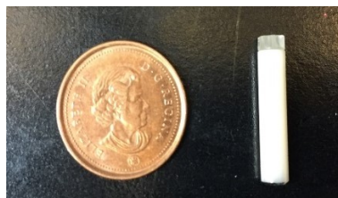
Figure 12. A 4 mm MAS rotor compared to a Canadian Penny for scale. The cap of the rotor is winged so that it may spin using a high pressure air stream. The spinning speed is adjusted using an MAS controller fit onto the spectrometer console.
