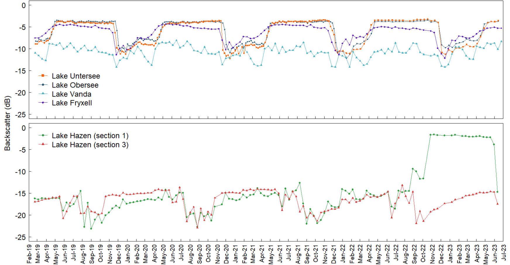
Fig. 13 Comparison of time series of SAR backscatter over lake ice. Time series of SAR backscatter (dB) over Lake Untersee, Lake Obersee, Lake Vanda, and Lake Fryxell (top) and two sections of Lake Hazen (bottom) between February 2019 and July 2023 in the descending trajectory. Delineations of sections 1 and 3 are the same as in Murfit & Duguay (2020) .
