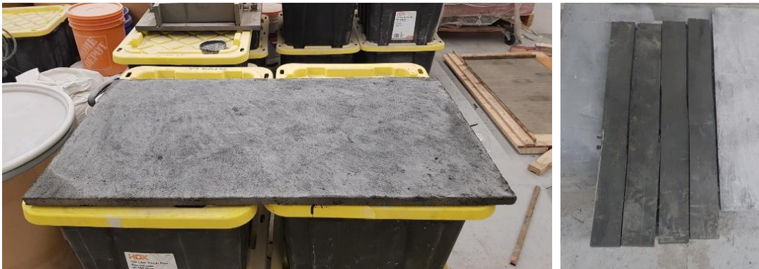
Figure 3-5: Rectangular panel of FRCM before cutting into coupons (left) and after cutting (right).
