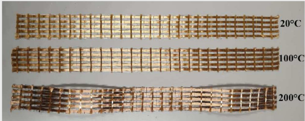
Figure 2-22: PBO-fabric after exposure to ambient and high temperature (Ombres et al. 2022).
