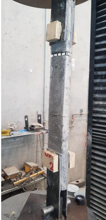
Figure 4-8: Crack development within the gauge length.
