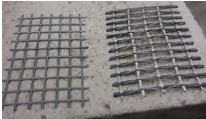
Figure 2-4: Unidirectional and bidirectional carbon grid (Simpson, 2020).
