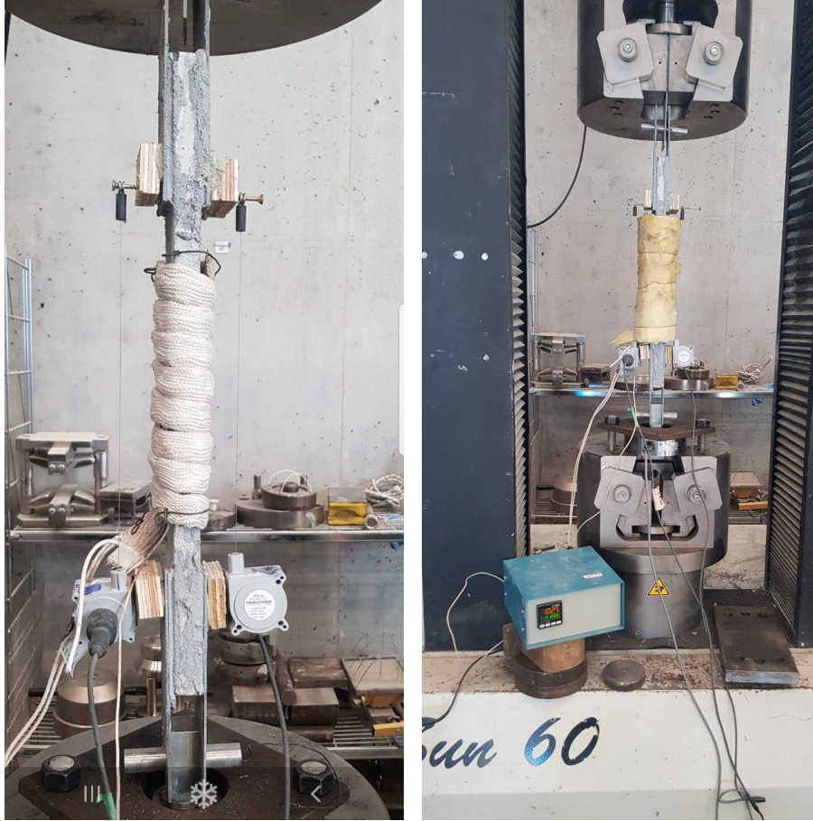
Figure 3-15: Loading test setup (left) before fibreglass wrapping and (right) after fibreglass wrapping.
