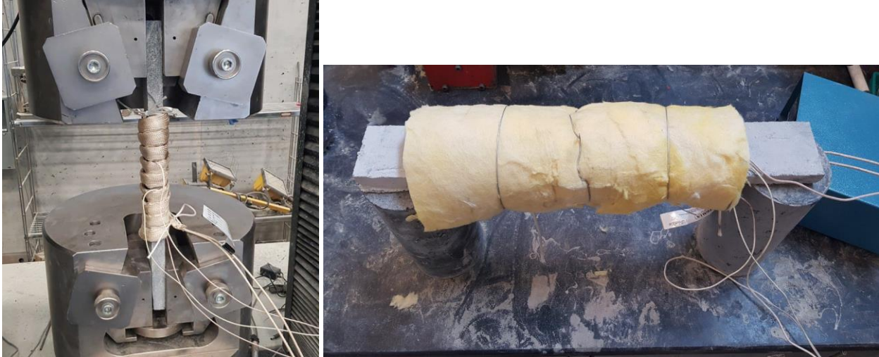
Figure 3-14: Heating test setup prior to insulating and after insulating.
