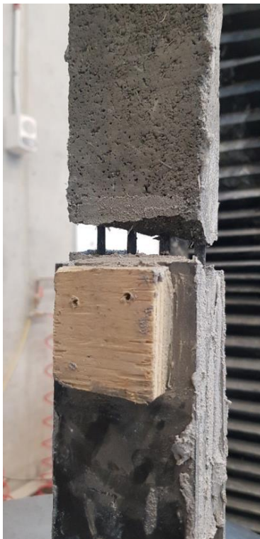
Figure 4-9: Fabric slippage within the surrounding matrix.
