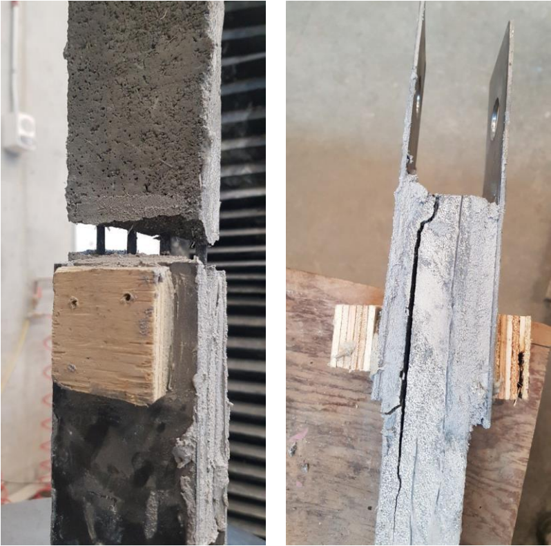
Figure 8-21: Failure modes of specimens, from left to right: slippage of fabric and debonding at fabric and matrix interface.
