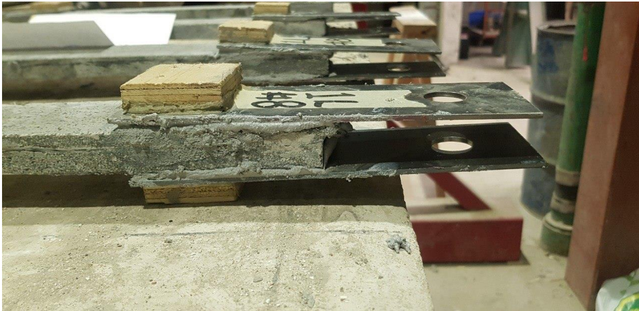
Figure 3-6: FRCM coupon with bonded steel tabs.
