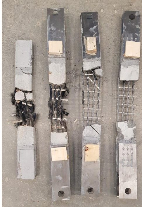
Figure 4-27: Fibre degradation due to high-temperature effect (left to right: 400, 300, 200, 100°C).
