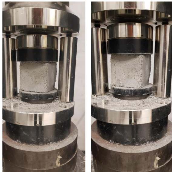
Figure 4-1: cubic cementitious matrix prior (left) and after the test (right).
