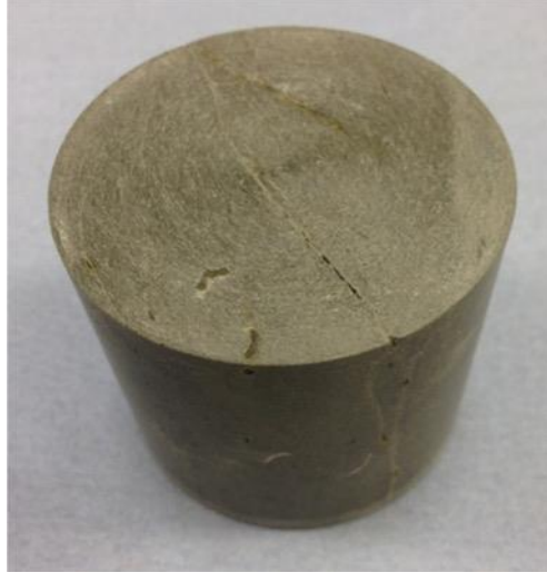
Figure 6.6 Naturally fractured COx-4 sample ( Harrington et al., 2017 )
