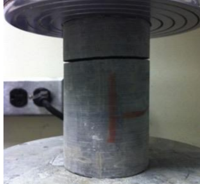
Figure 5.13 Failure characteristics after uniaxial tension test ( Gao et al., 2015 )
