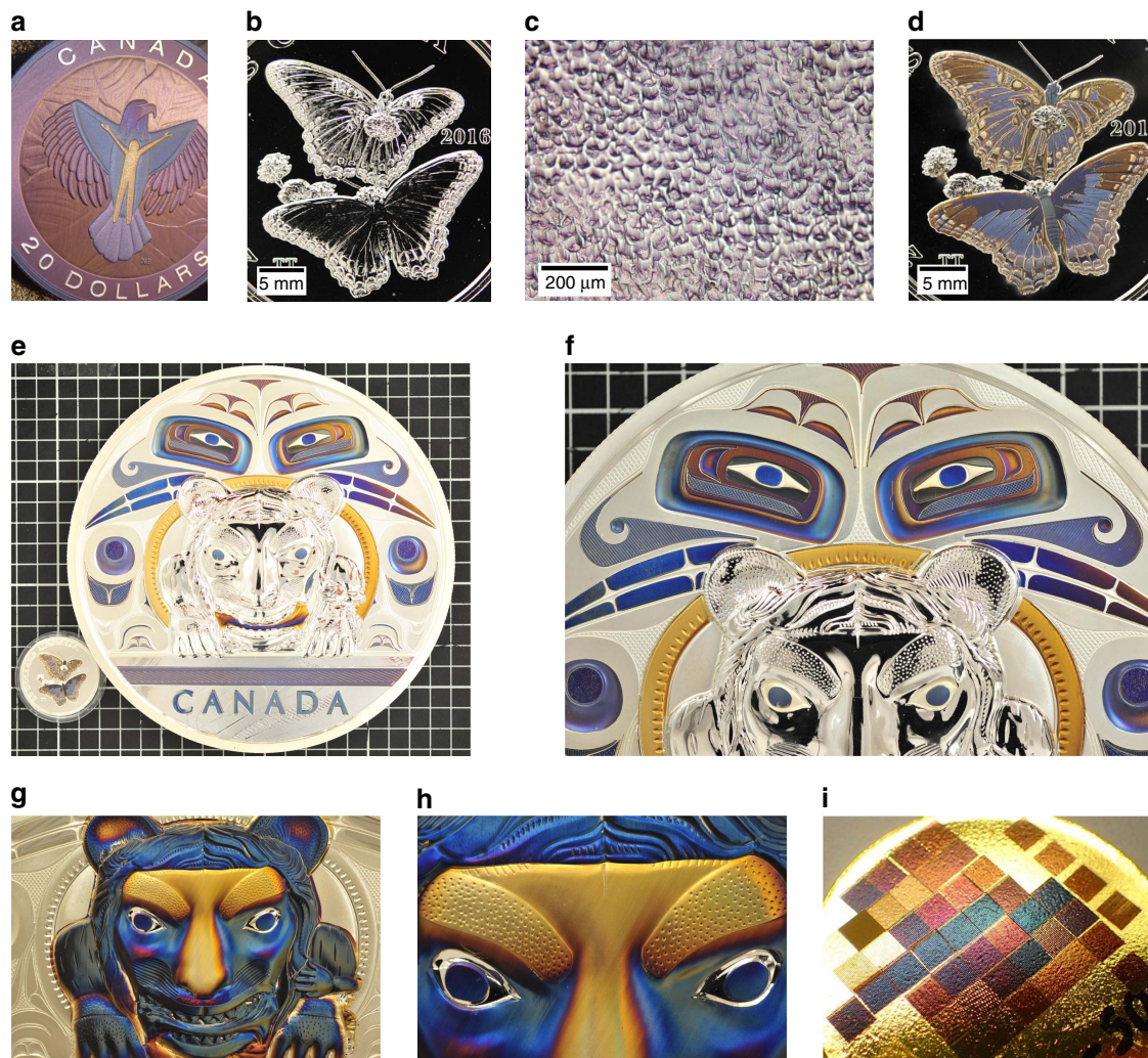
Figure 1 | Laser colouring of large areas having significant topographic variations. (a) Photograph of a coloured silver coin featuring a representation of an eagle. (b,d) Photographs of silver coins bearing a frosted butterfly (b) before and (d) after laser colouring. The topography on these coins has an overall height of \sim 2 mm. The distinctive white areas on the butterfly are due to the frosted (that is, melted) finish; (c) optical microscope image of the frosted regions, having topographic variations of up to 2 mm in height and a roughness of \sim 1 to 2 \mu\text{m} . (e) Photograph of a laser-coloured 5 kg silver coin of diameter 21 cm and thickness 2.5 cm (the butterfly coin of (d) is also shown for comparison). (f) Close-up of (e) showing crevices \sim 5 mm deep of black-and-white-coloured eyes. (g) Alternate colouring of another 5 kg coin over topographic relief \sim 1 cm in height. (h) Close-up of (g) near the nose and brow, the highest points on the coin. (i) Angle-independent colours produced on the surface of a gold coin.
