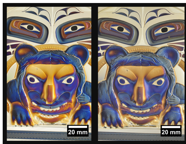
Figure 11. Pre (left) and post (right) ALD of alumina on a sample (two-step ALD process). Photograph of a laser colored 5 kg collectible silver sample before (left) and after (right) the two-step ALD of a composite alumina passivation film (porous and dense) 15 nm thick.
