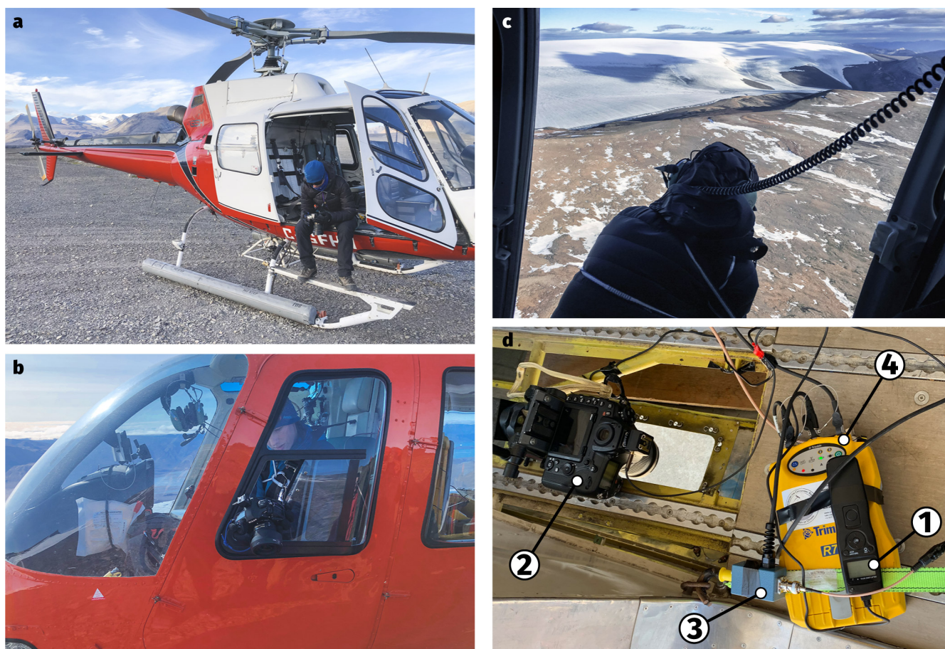
Figure 3.3. Camera position onboard the helicopter during the [a] TF and [b] EF surveys. [c] Image capture during the TF survey, and [d] imaging/positioning hardware used at both TF and EF (shown here as used in another survey not part of this study): (1) intervalometer; (2) Nikon D850 camera; (3) Trimble event marker device; (4) Trimble R7 GPS receiver.
