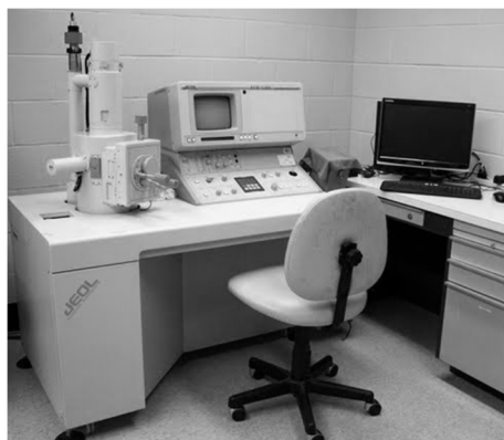
Figure 3-16: JEOL JSM-5300 Scanning Electron Microscope (SEM); Resolution: 10-20 nm, Magnification: high vacuum mode 15x-200,000x and low vacuum mode 15x-50,000x, Acceleration voltage: 0.5-30 kV, Specimen size: up to 76 mm in diameter.
