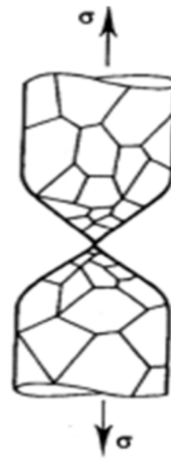
Figure 4-13: Ductile fracture mode by 100% reduction in area
