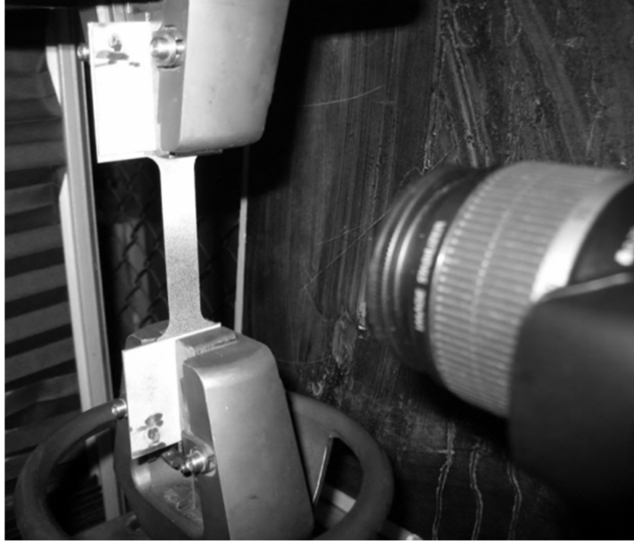
Figure 3-20: Pre-strain test setup; using tensile machine (Instron 4482) and taking picture during the test with digital camera
