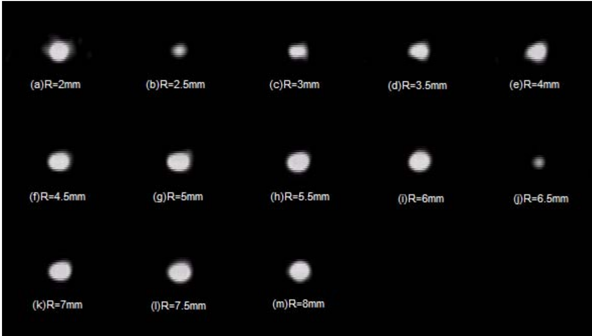
Figure 3.4: Mosaic of mode outputs of S-bends of different radii of curvature
