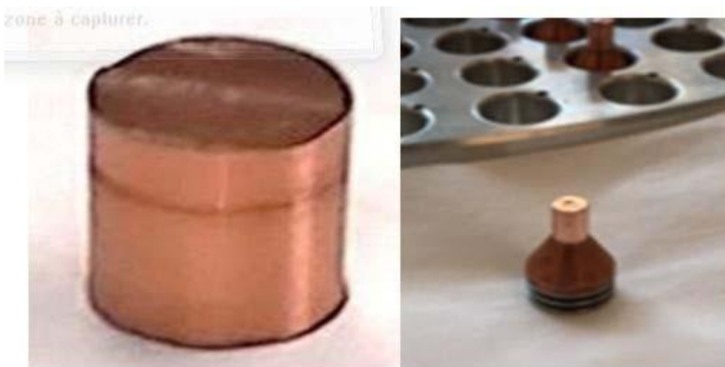
Figure 14: (left image) Target, (right image), mounted on the target base (below) and loaded in the ion source "wheel" (top).
