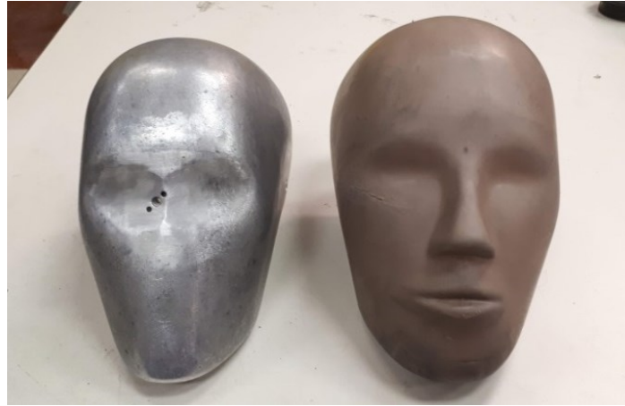
Figure 4. The Hybrid III headform separated to reveal the interior steel structure (left) and external vinyl skin (right).
