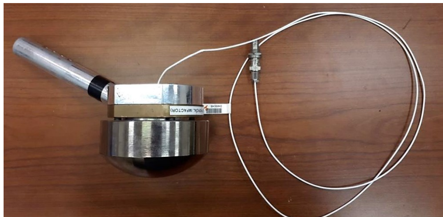
Figure C-1. Spherical impactor instrumented with one uniaxial accelerometer.
