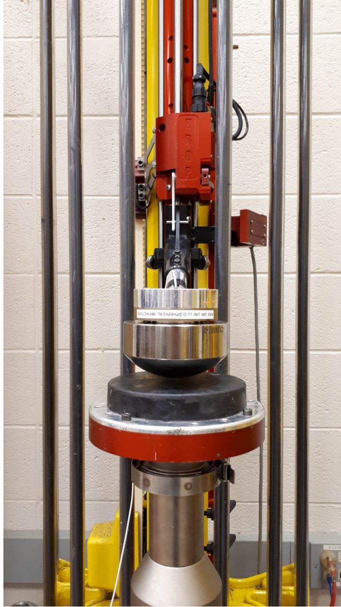
Figure C-2. Monorail drop rig with spherical impactor, uniaxial accelerometer, and MEP pad.
