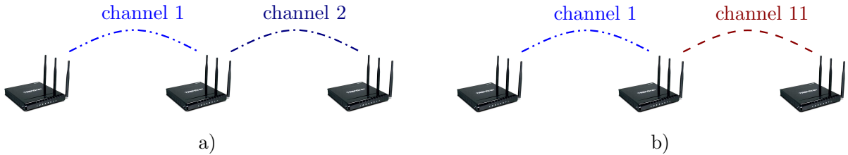
Figure 2.7: In a), two overlapping Wi-Fi channels produce cross-channel interference, whereas in b), two Wi-Fi orthogonal channels do not.
