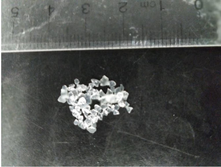
Figure 2-13. Photo of crushed silica gel sieved to 12-20 mesh size.
