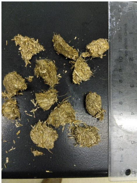
Figure 2-10. Photo of flax shive briquette pieces.
