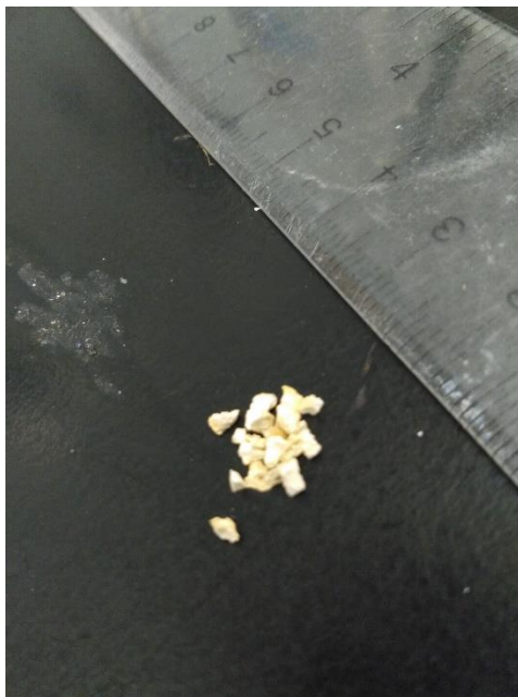
Figure 2-9. Photo of crushed titanium silicate molecular sieve particles sieved to 12-20 mesh size.
