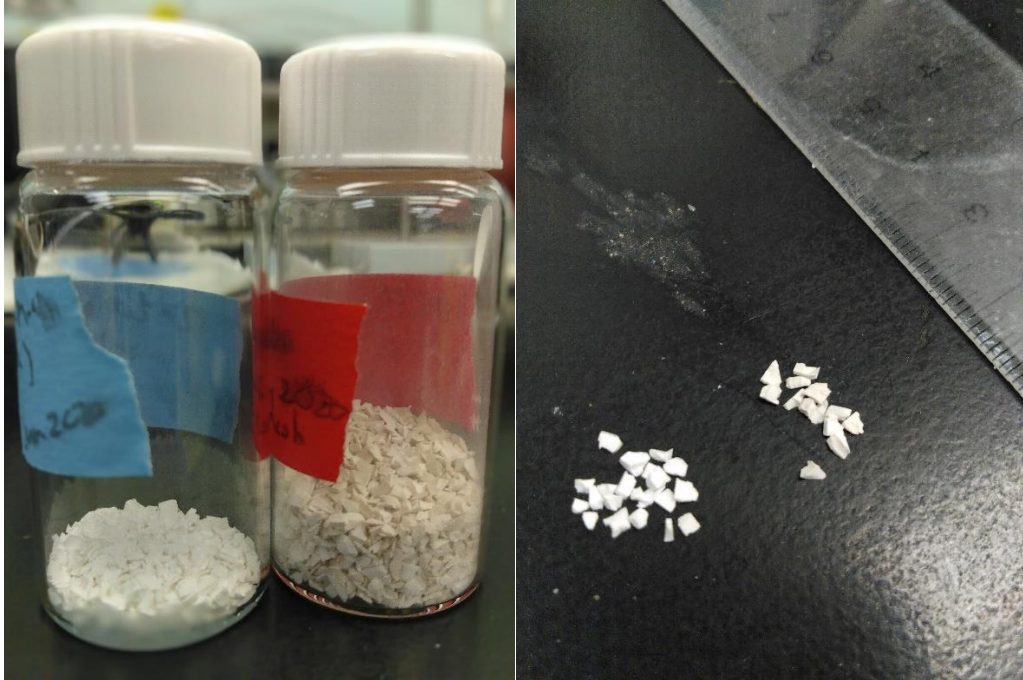
Figure 2-11. Photo of crushed MCM-41 particles sieved to 12-20 mesh size before (left) and after (right) lab-scale energy storage testing.
