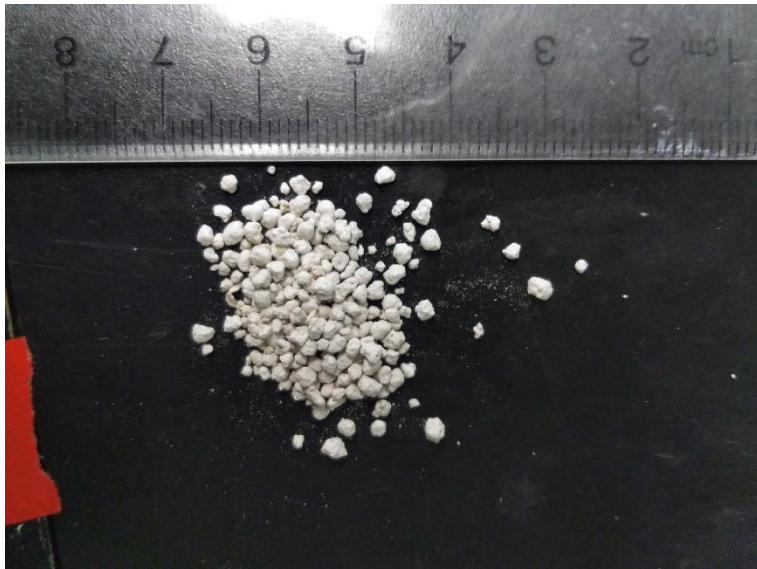
Figure 2-12. Photo of spherical SAPO-34 pellets.
