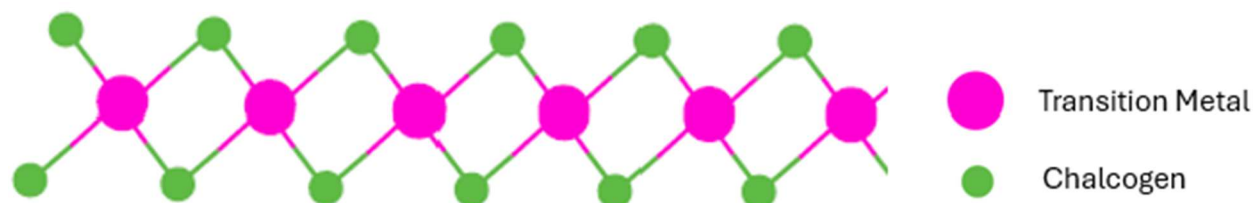
Figure 2.4: Atomic structure representation of Transition Metal Dichalcogenides (sideview), where the middle plane is the transition metal and the top-bottom planes are chalcogens.
