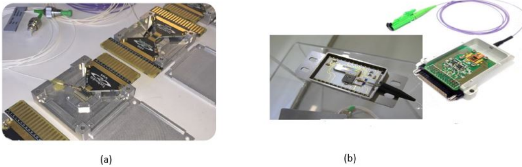
FIGURE 6.2: (a) Standard package from Technobis (Tipps) for photonic integrated circuits. (b) A customized package from the same company. Their PDK is available through Phoenix design kit
