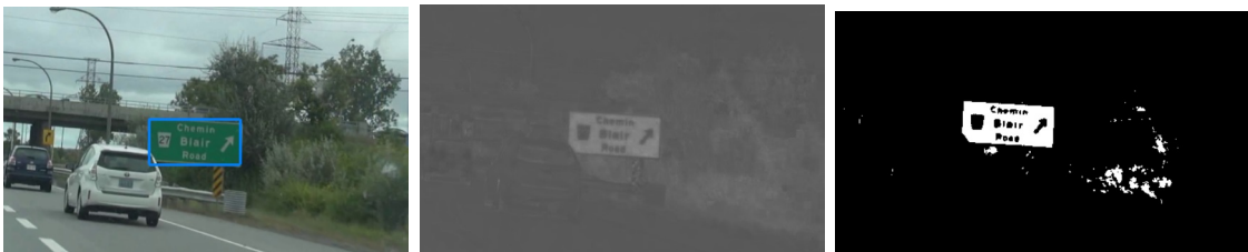
Figure 3.10: Left: original frame, Mid: green-normalized frame, Right: thresholded frame
