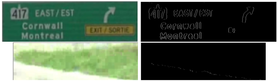
Figure 3.14: Top: A traffic board and its canny-edge equivalent, Bottom: An unwanted object and its canny-edge equivalent
