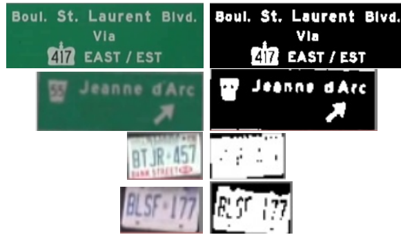
Figure 3.9: Through observation, we were able to deduce that our OOIs exhibit a fixed range of white to non-white pixel ratios
