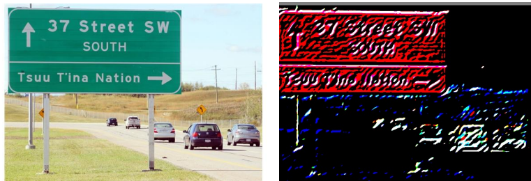
Figure 2.8: Left: Original Image, Right: Output with Gabor filter
