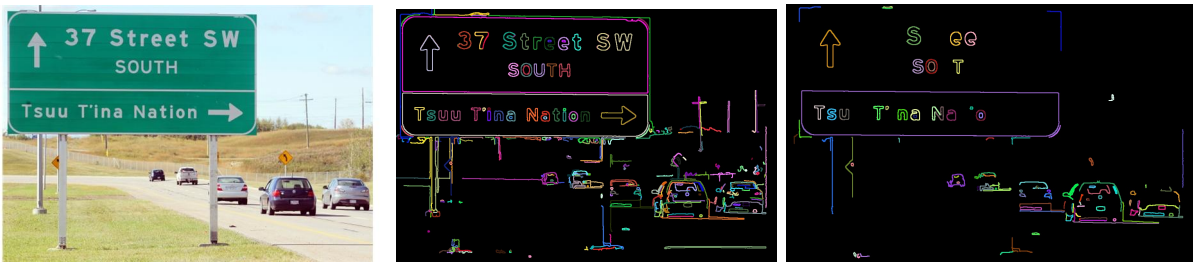
Figure 2.4: Left: Original Image, Middle: Output with Canny edge detector, Right: Output with Canny edge detector + threshold
