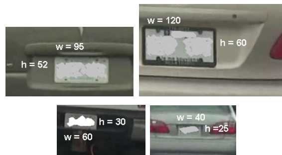
Figure 3.5: An example of how we determined the dimension constraints for license plates (sizes are in pixels from a 900 \times 600 frame)
