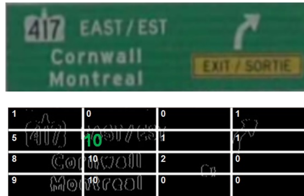
Figure 5.1: Maximum cell (10) > t_{max} and is adjacent to cells containing > t_{avg} cells \Rightarrow First condition satisfied
