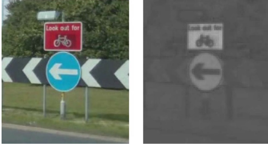
Figure 2.7: Left: Original image, Right: Red-Blue Normalized image, taken from [35]
