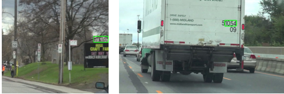
Figure 5.11: Sample false positives in detecting LPs. For such a false positive to occur, the false region must be edge-heavy as well as be surrounded by edge-light areas so that it passes all texture filters. Additionally, to pass the color filter, it must exhibit a certain ratio of white to non-white pixels
