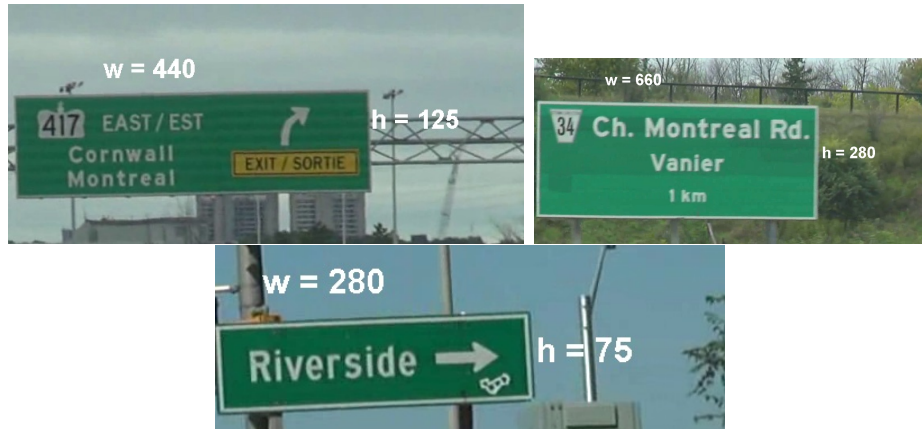
Figure 3.4: An example of how we determined the dimension constraints for traffic boards (sizes are in pixels from a 900 \times 600 frame)
