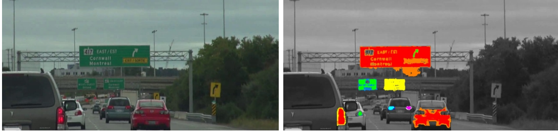
Figure 3.3: Left: original frame, Right: same frame with the MSERs highlighted
