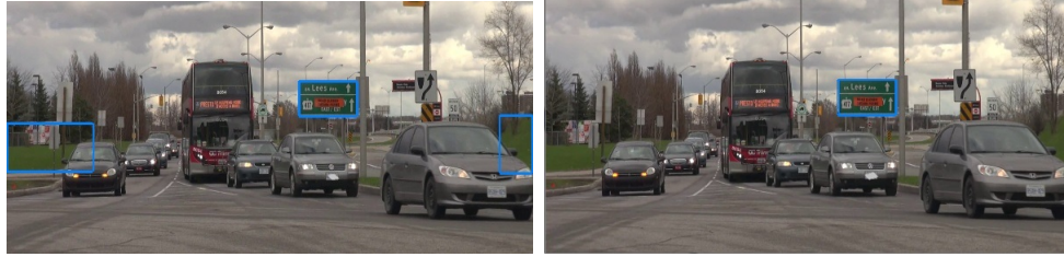
Figure 3.12: Left: sample frame before applying the color filter, Right: same frame after applying the color filter. The color filter is also able to remove false positives that contain green pixels if they do not satisfy a color threshold. Details on this threshold are provided in Section 5.2.1.
