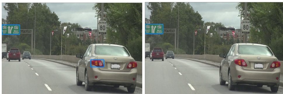
Figure 3.11: Left: sample frame before applying the color filter, Right: same frame after applying the color filter. The false positive present in the first frame is removed by the color filter due to the absence of green pixels.
