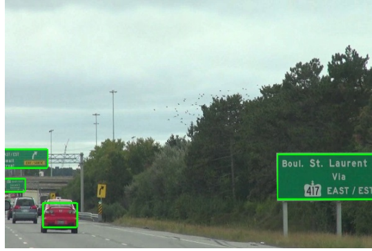
Figure 3.7: Attempting to detect objects from all ranges could result in false positives
