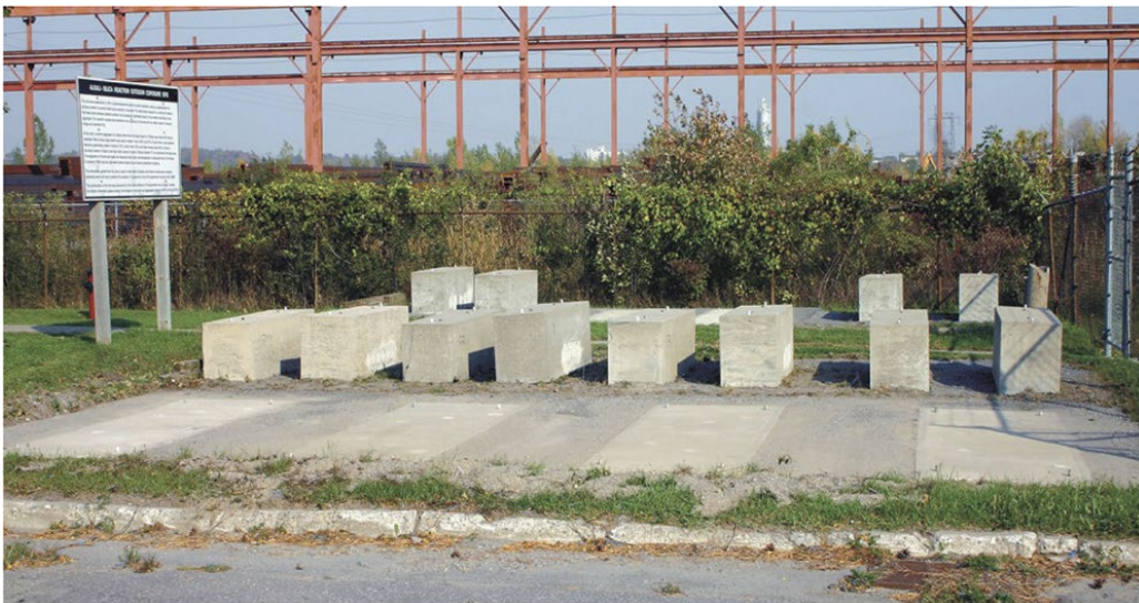
Figure 4.12: Beams from Kingston exposure site for ASR [41].
