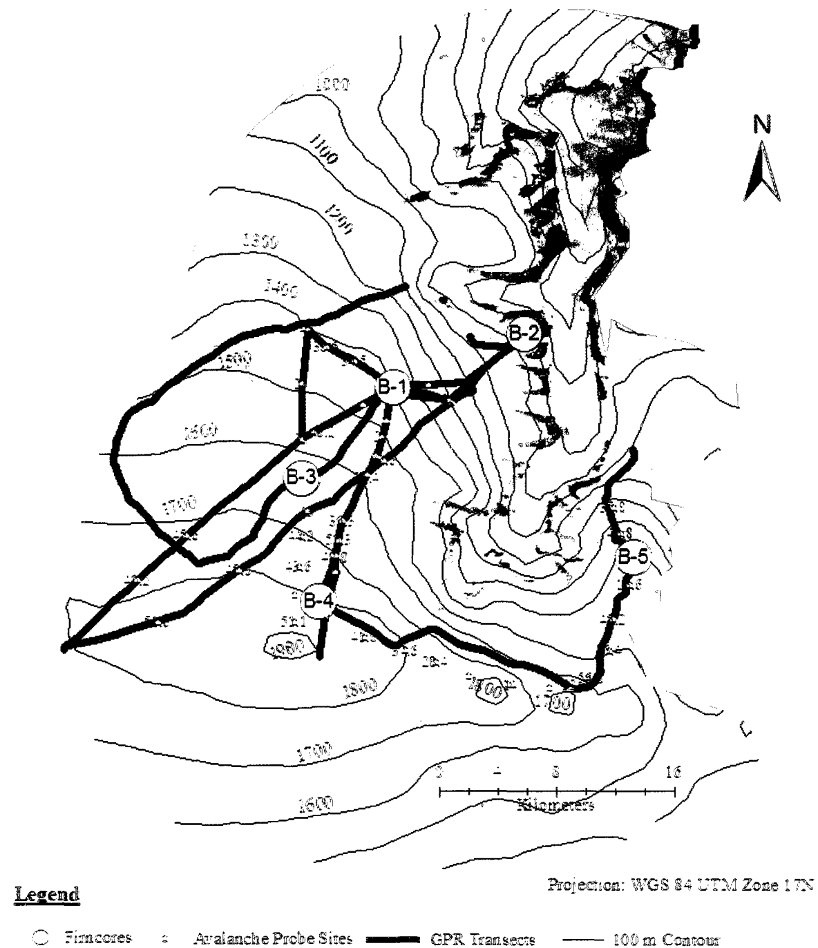
Figure 3.3. GPR transects, avalanche probe, and shallow borehole measurements for 2008 field season (Base image: Landsat 7, July 7, 2000).
