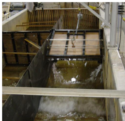
Figure 4.1- Experimental setup of Al-Faesly et al. [2013] showing the generation of a turbulent hydraulic bore [Al-Faesly et al. , 2012]
