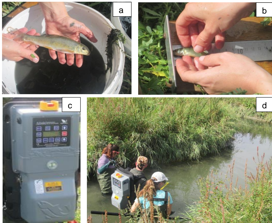
Figure 5.5. Fish sampling survey in the study reach: (a) Fish were hold in the bucket till they were measured and identified (b) Measurement and identification of the caught fish (c) Backpack electrofisher (d) Fish sampling in the study reach using backpack electrofishing (R-L: J. Foster, C.K. Elvidge, K. Birnie-Gauvin).
