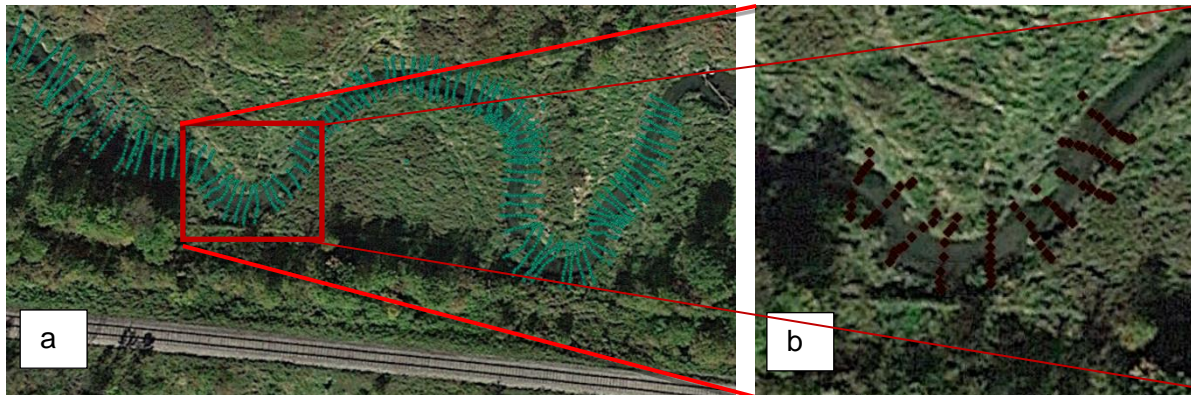
Figure 5.2. Total station bathymetric points collected during summer: (a) 2014 (b) 2016. Flow from left to right. Background pictures taken from Google Earth.
