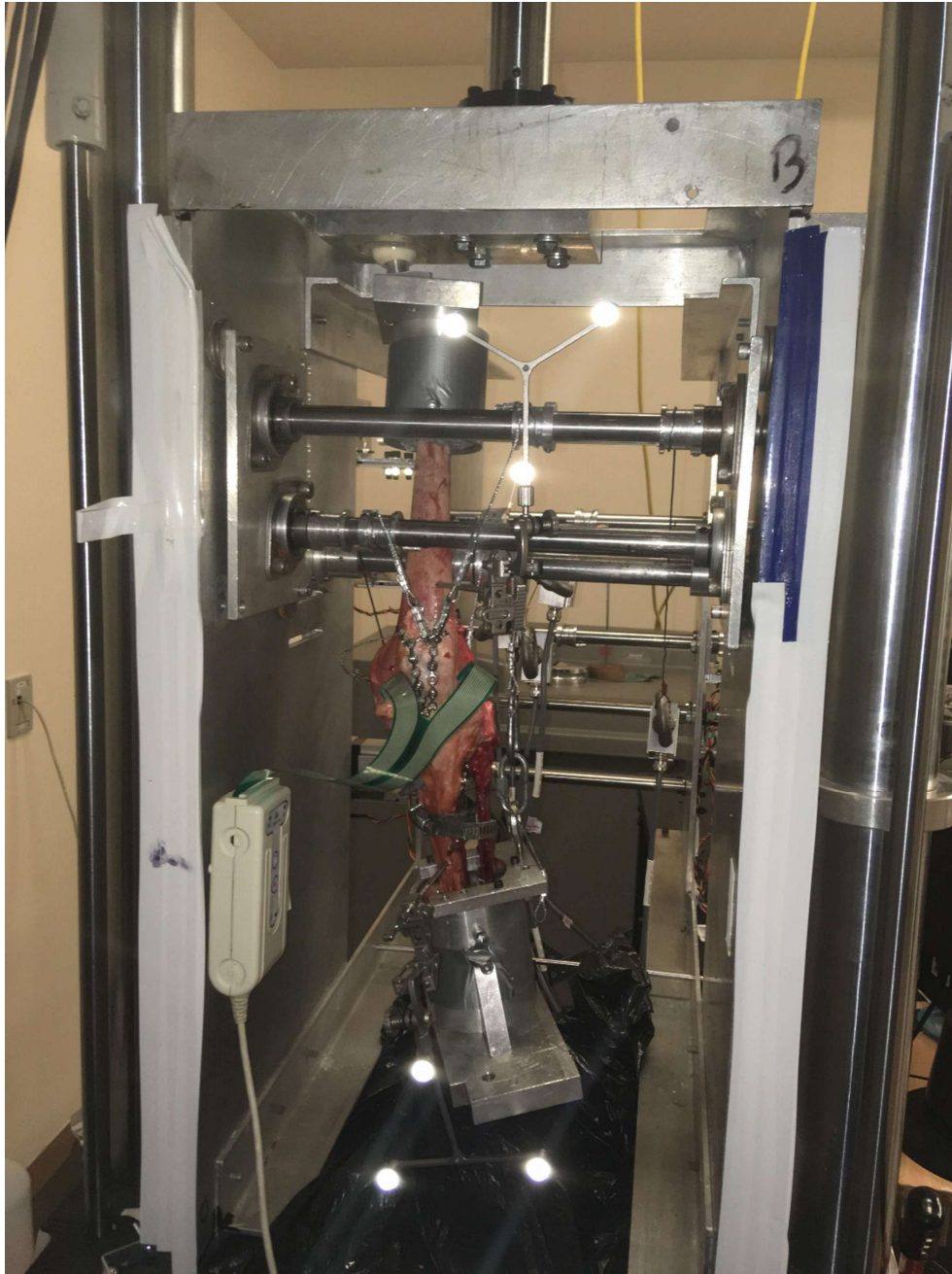
Figure 17. UOKS with specimen suspended. Bone pins were used to fix the Polaris tracking tools to each segment. Tekscan sensor inserted inside the knee joint.
